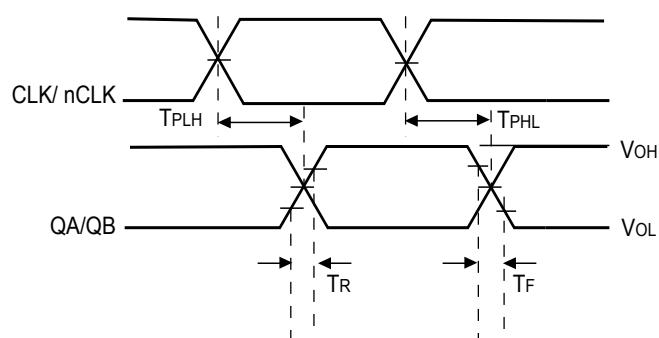
$$T_{SK} = T_{PLH2} - T_{PLH1} \text{ or } T_{SK} = T_{PHL2} - T_{PHL1}$$
