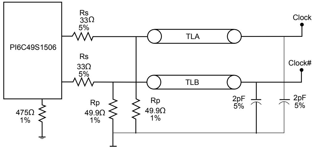
**Configuration Test Load Board Termination for LVPECL/ LVDS**
