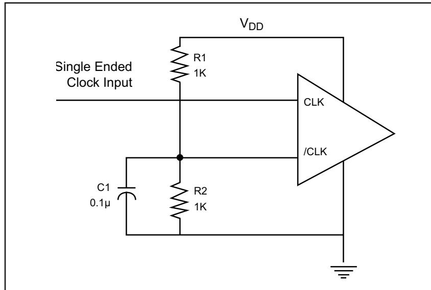
Figure 1. Single-ended input to Differential input device
