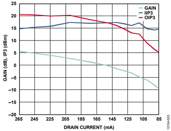
Figure 28. Gain and Input/Output IP3 vs. Drain Current,  $P_{IN} = -5$  dBm/Tone,  $V_{CTL1}/V_{CTL2} = -1$  V, RF = 86 GHz, Drain Current = ( $I_{DD1}/I_{DD2}$  Fixed at 50 mA) + ( $I_{DD3}$  to  $I_{DD6}$  Swept)
