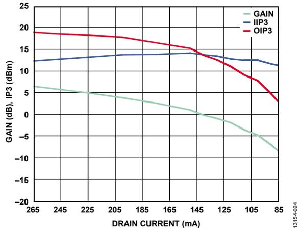
Figure 26. Gain and Input/Output IP3 vs. Drain Current,  $P_{IN} = -5$  dBm/Tone,  $V_{CTL1}/V_{CTL2} = -1$  V, RF = 81 GHz, Drain Current = ( $I_{DD1}/I_{DD2}$  Fixed at 50 mA) + ( $I_{DD3}$  to  $I_{DD6}$  Swept)
