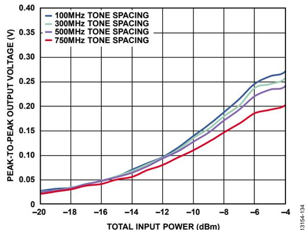
Figure 34. Envelope Detector Peak-to-Peak Output Voltage vs. Total Input Power at Various Tone Spacings, RF = 81 GHz,  $V_{CTL1}/V_{CTL2} = -5$  V,  $V_{DET} = 4$  V with 150  $\Omega$  Load Impedance at  $ENV_{DET}$
