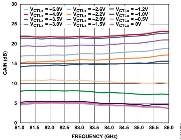
Figure 12. Gain vs. Frequency at Various Control Voltages
