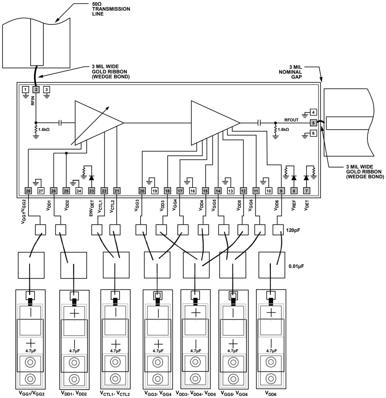
Figure 39. Assembly Diagram
