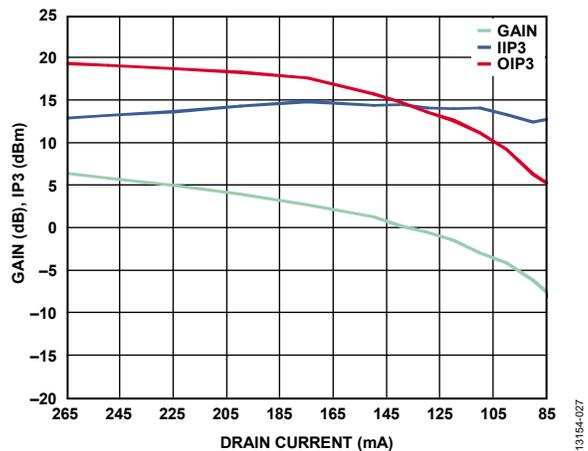
Figure 27. Gain and Input/Output IP3 vs. Drain Current,  $P_{IN} = -5$  dBm/Tone,  $V_{CTL1}/V_{CTL2} = -1$  V, RF = 83.5 GHz, Drain Current = ( $I_{DD1}/I_{DD2}$  Fixed at 50 mA) + ( $I_{DD3}$  to  $I_{DD6}$  Swept)
