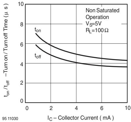
Figure 14. Turn on / off Time vs. Collector Current
