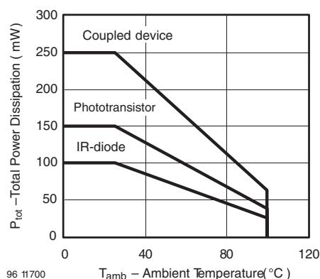
Figure 6. Total Power Dissipation vs. Ambient Temperature
