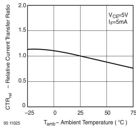
Figure 8. Relative Current Transfer Ratio vs. Ambient Temperature
