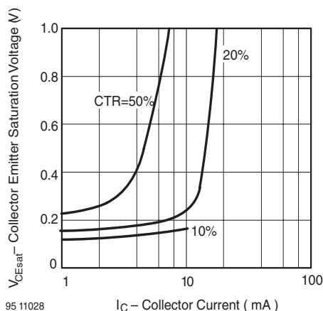
Figure 12. Collector Emitter Saturation Voltage vs. Collector Current
