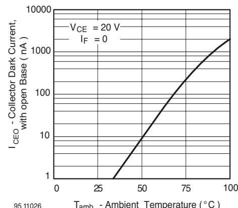
Figure 9. Collector Dark Current vs. Ambient Temperature
