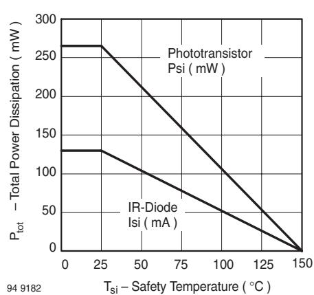
Figure 1. Derating diagram
