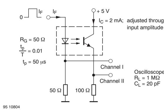
Figure 3. Test circuit, non-saturated operation
