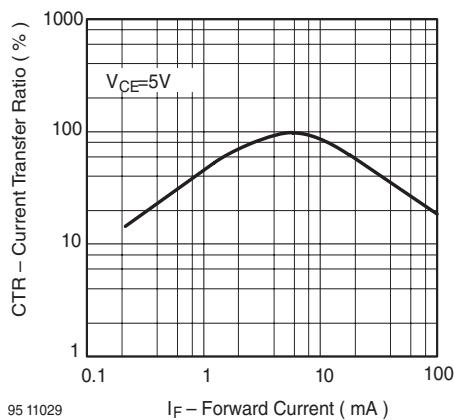
Figure 13. Current Transfer Ratio vs. Forward Current
