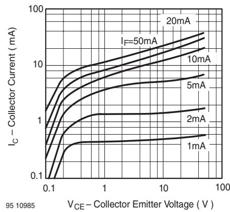
Figure 11. Collector Current vs. Collector Emitter Voltage
