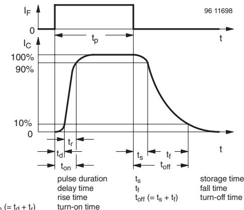
Figure 5. Switching Times
