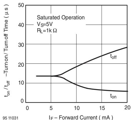
Figure 15. Turn on / off Time vs. Forward Current
