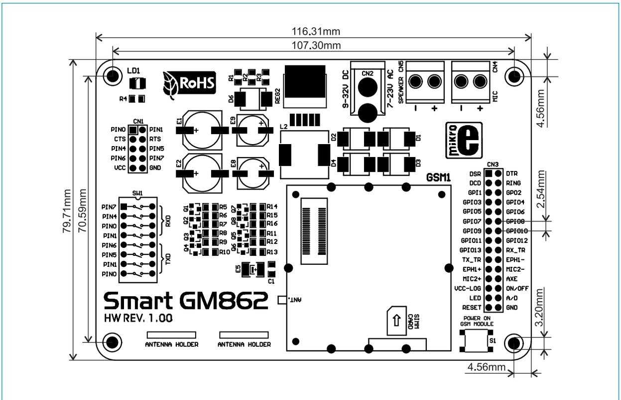
Figure 3: SmartGM862 dimensions
