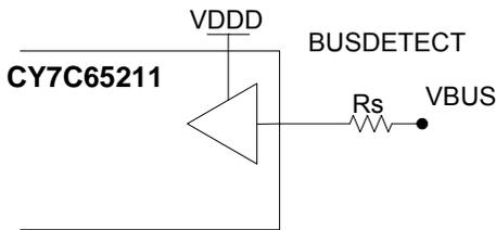
When the VBUS > VDD, a resistor voltage divider is required to reduce the voltage from the VBUS down to VDD for the GPIO sensing the VBUS voltage. This is shown in the following figure. The resistors should be sized as follows:
