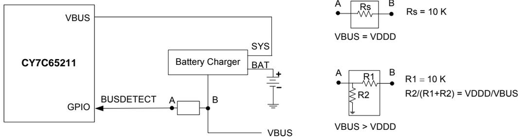
When the VBUS and VDD are at the same voltage potential, the VBUS can be connected to the GPIO using a series resistor ( $R_s$ ). This is shown in the following figure. If there is a charger failure and the VBUS becomes 9 V, then the 10-k $\Omega$  resistor plays two roles. It reduces the amount of current flowing into the forward-biased diodes in the GPIO, and it reduces the voltage seen on the pad.
