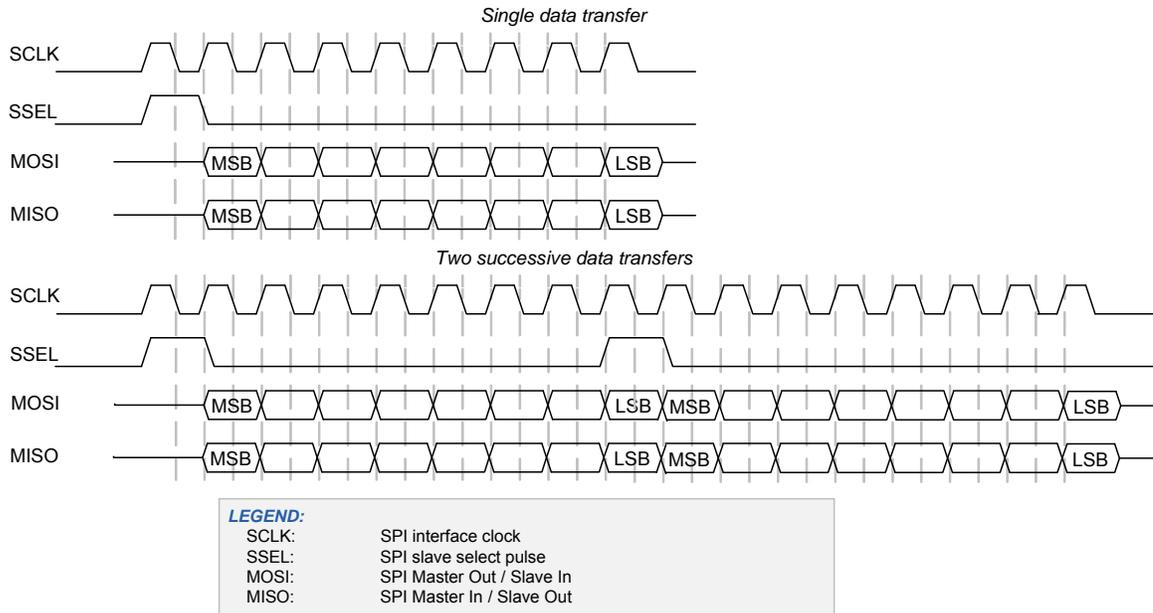
The following figure illustrates a single 8-bit data transfer and two successive 8-bit data transfers. The SSEL pulse coincides with the first data bit.
