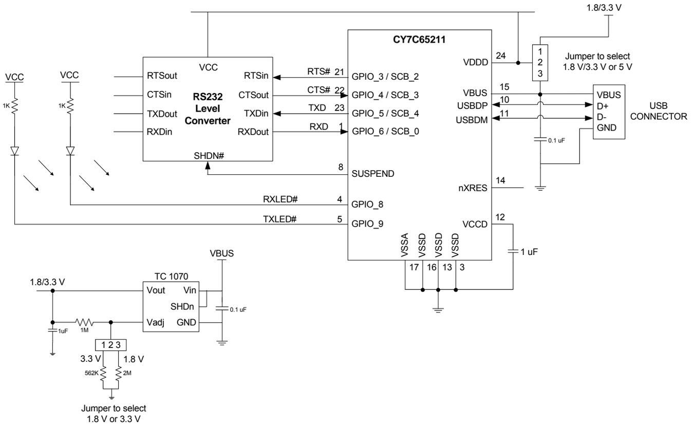
In a battery charger system, a 9-V spike on the VBUS is possible. The CY7C65211 VBUS pin is intolerant to voltage above 6 V. In the absence of over-voltage protection (OVP) on the VBUS line, the VBUS should be connected to BUSDETECT (GPIO configured) using the resistive network and the output of the battery charger to the VBUS pin of CY7C65211, as shown in the following figure.
