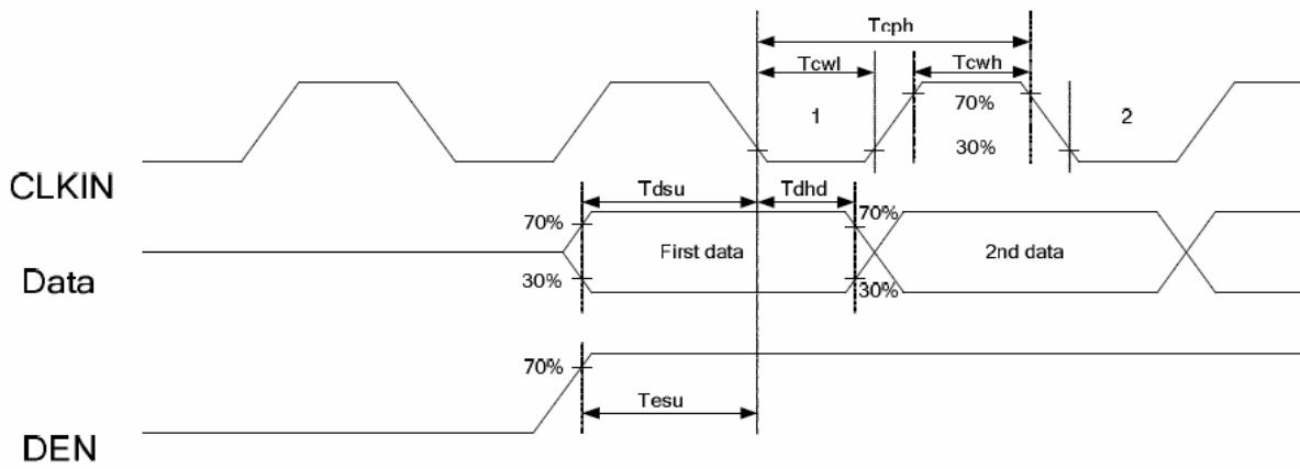
Figure 3:Pixel Timing
