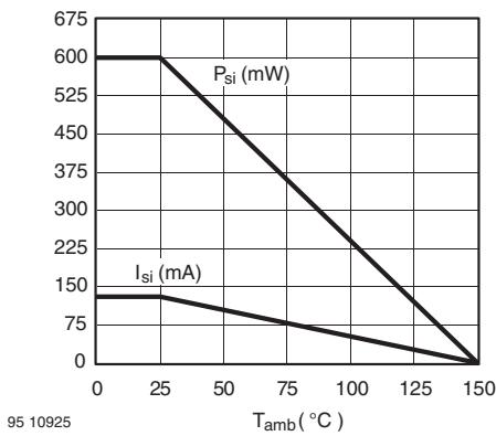
Figure 4. Derating diagram
