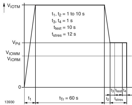
Figure 5. Test pulse diagram for sample test according to DIN EN 60747-5-2(VDE0884)/ DIN EN 60747-5-5 pending
