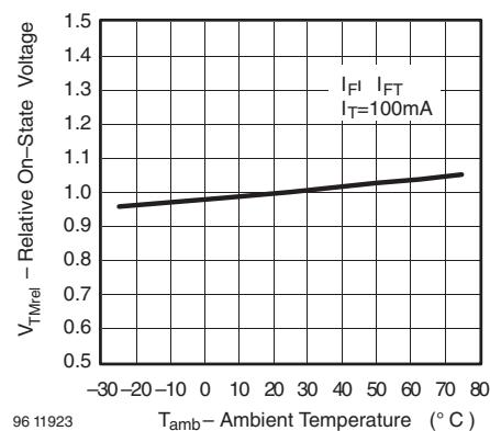
Figure 9. Relative On - State vs. Ambient Temperature
