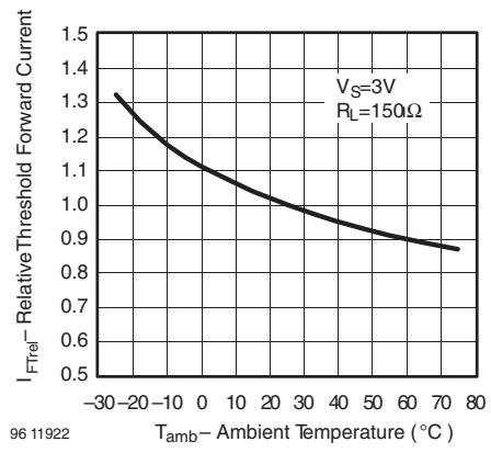
Figure 8. Relative Threshold Forward Current vs. Ambient Temperature
