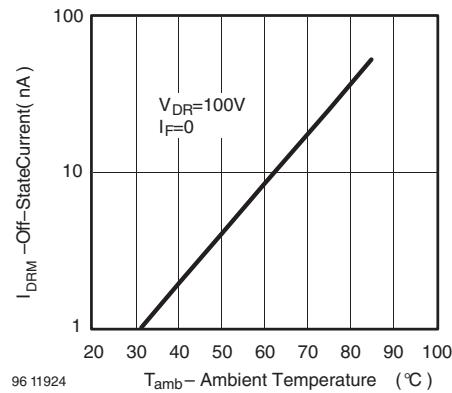
Figure 10. Off - State Current vs. Ambient Temperature
