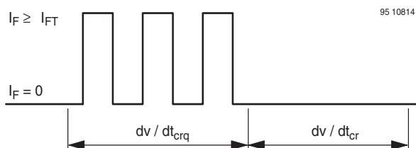
$dV/dt_{cr}$  Highest value of the "rate of rise of off-state voltage" which does not cause any switching from the off-state to the on-state
