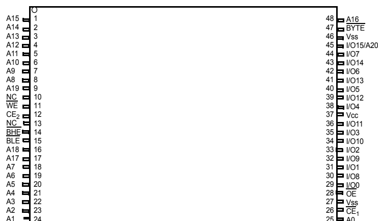
Figure 2. 48-pin TSOP I pinout (Top View) [2, 3]
