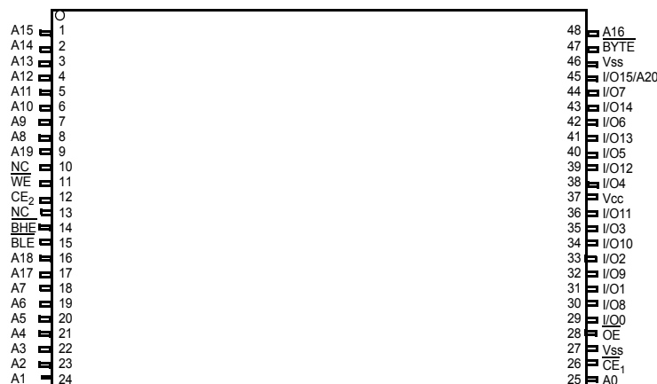
Figure 2. 48-pin TSOP I pinout (Top View) [2, 3]
