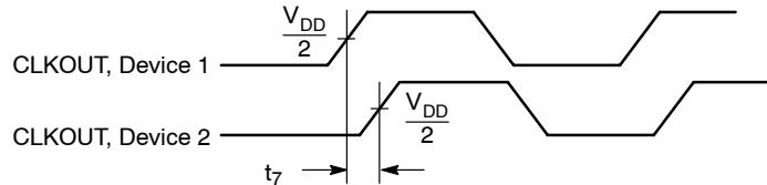
**Figure 7. Device – Device Skew**
