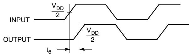
**Figure 6. Input – Output Propagation Delay**
