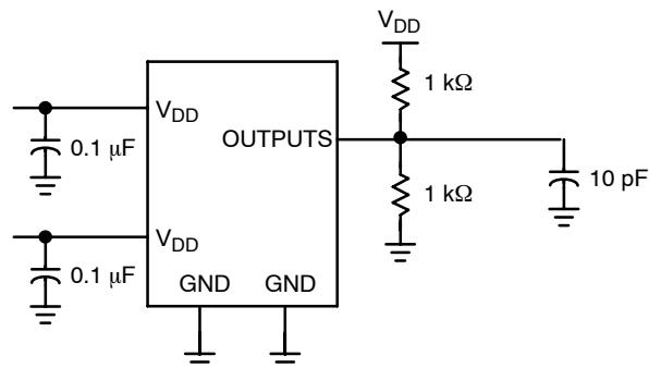
**Figure 9. Test Circuit #2**
