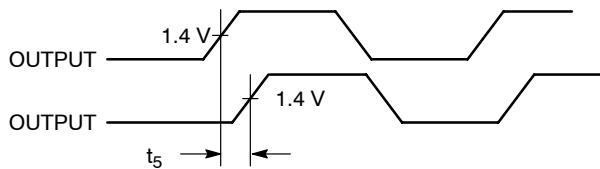
**Figure 5. Output – Output Skew**
