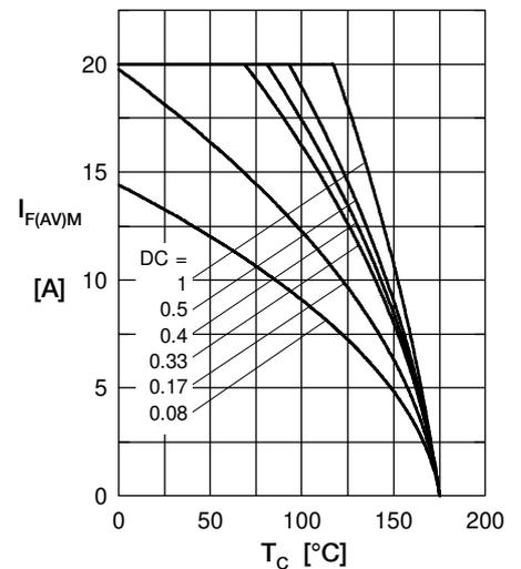
Fig. 5 Max. forward current vs. case temperature
