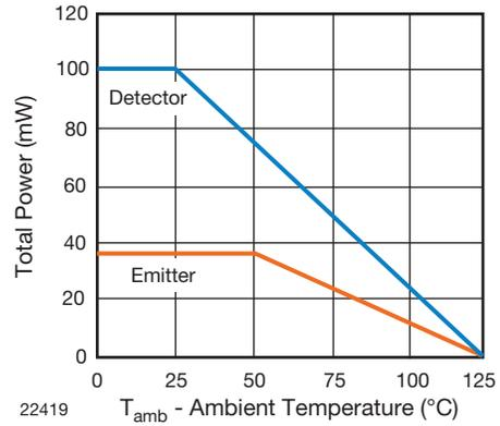
Fig. 3 - Permissible Power Dissipation vs. Temperature
