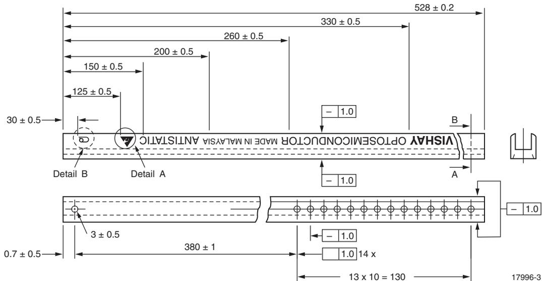
Fig. 4 - Shipping Tube Specifications for DIP-8 Packages
