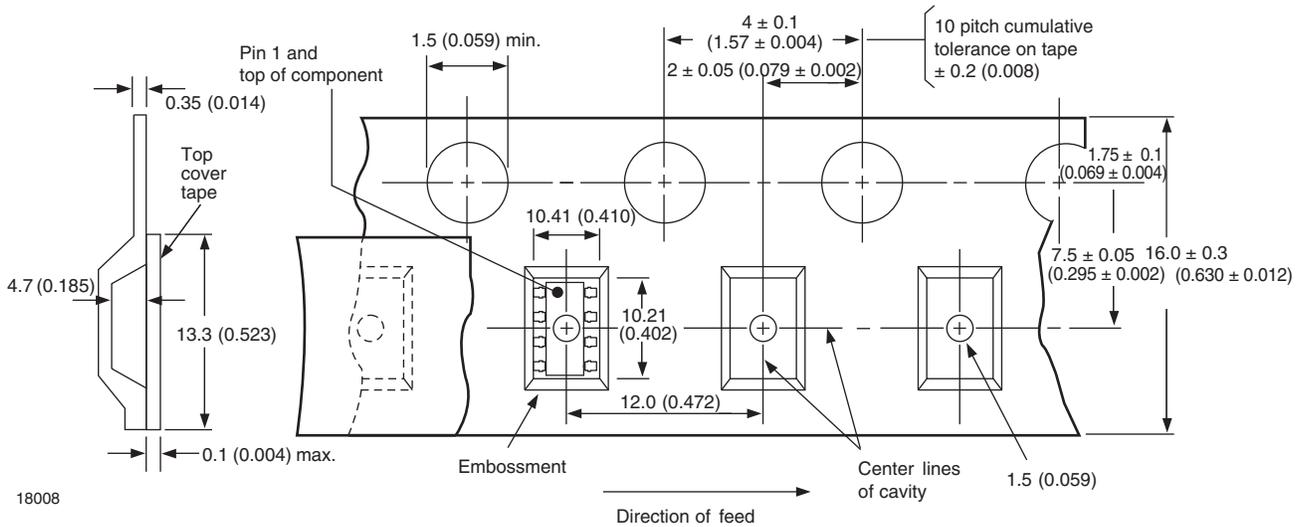
Fig. 8 - Tape and Reel Packing (1000 pieces on Reel)
