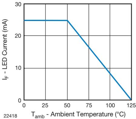
Fig. 2 - Permissible Forward LED Current vs. Temperature
