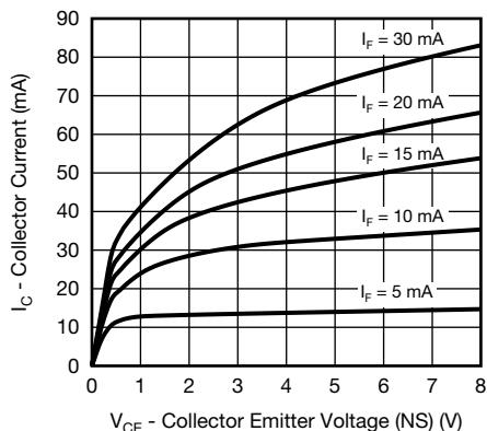
Fig. 5 - Collector Current vs. Collector Emitter Voltage (NS)
