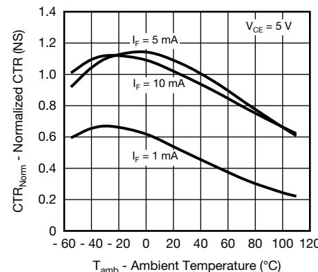
Fig. 8 - Normalized CTR (NS) vs. Ambient Temperature
