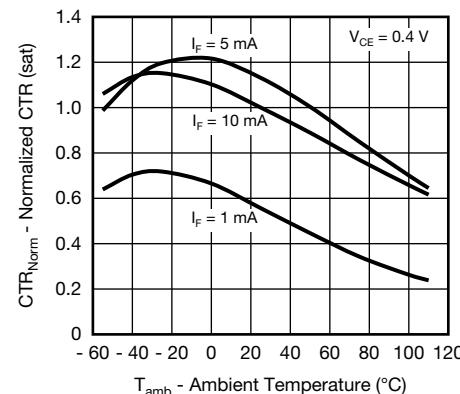
Fig. 9 - Normalized CTR (sat) vs. Ambient Temperature
