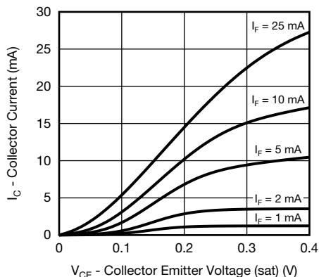
Fig. 6 - Collector Current vs. Collector Emitter Voltage (sat)
