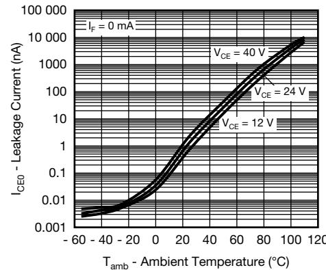
Fig. 7 - Leakage Current vs. Ambient Temperature
