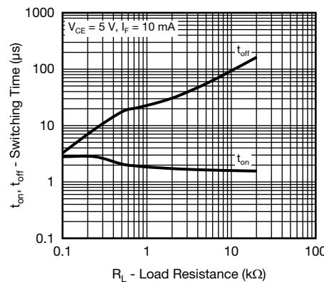
Fig. 14 - Switching Time vs. Load Resistance
