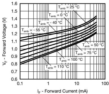
Fig. 4 - Forward Voltage vs. Forward Current
