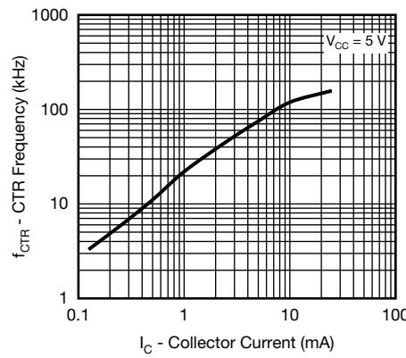
Fig. 13 - CTR Frequency vs. Collector Current
