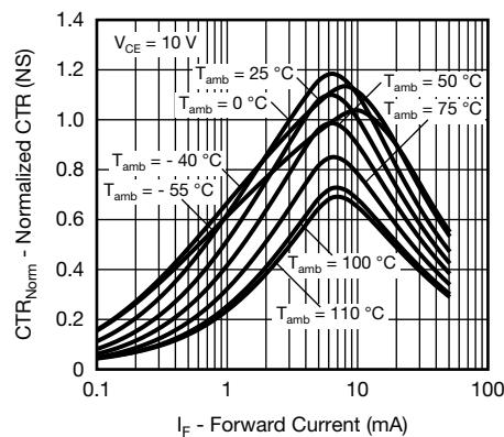
Fig. 10 - Normalized CTR (NS) vs. Forward Current
