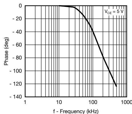
Fig. 12 - CTR Frequency vs. Phase Angle
