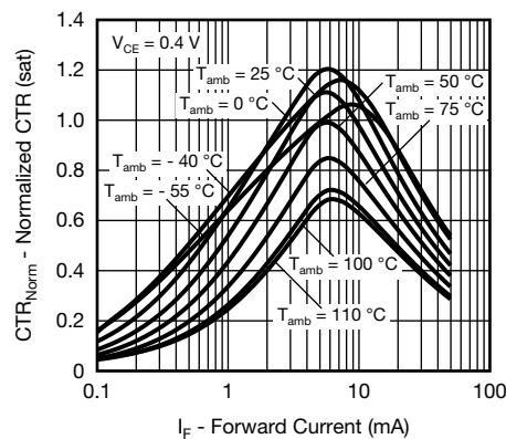
Fig. 11 - Normalized CTR (sat) vs. Forward Current
