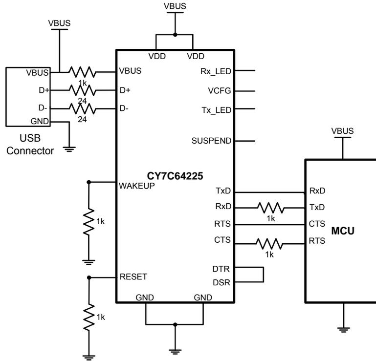
**Interfacing CY7C64225 with Self Powered Microcontroller**
