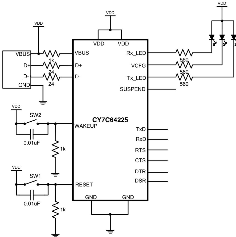
**Bus Powered Design using External Regulator**
