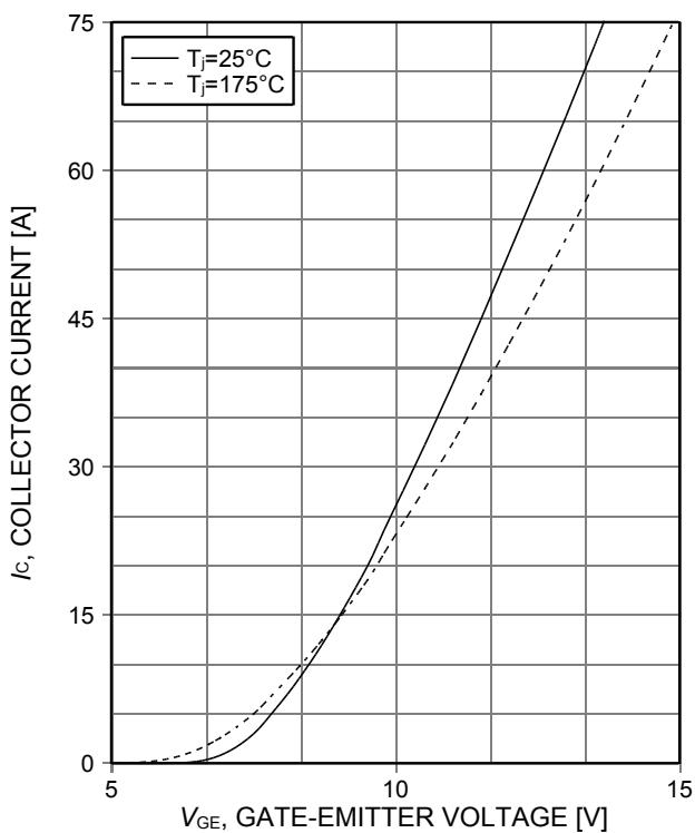
**Figure 7. Typical transfer characteristic**
