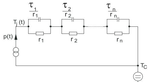
Figure D. Thermal equivalent circuit
