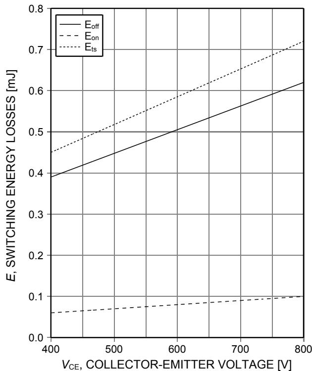
Figure 4. **Typical switching energy losses as a function of collector-emitter voltage**
