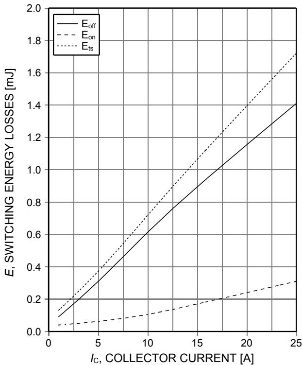
Figure 1. **Typical switching energy losses as a function of collector current**
