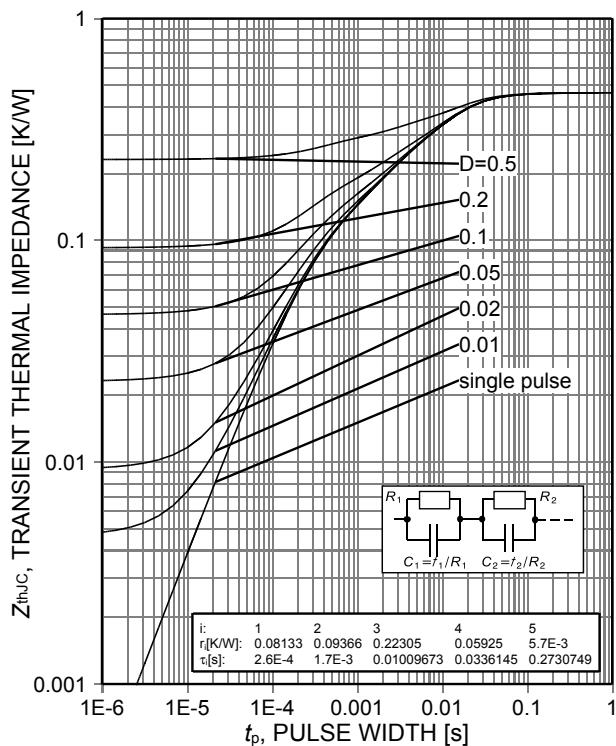
Figure 21. IGBT transient thermal impedance
