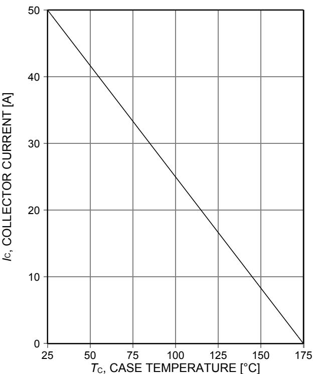
**Figure 4. Collector current as a function of case temperature**
