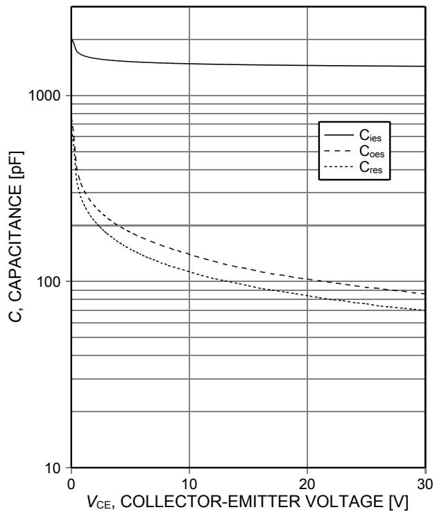
Figure 18. **Typical capacitance as a function of collector-emitter voltage**
