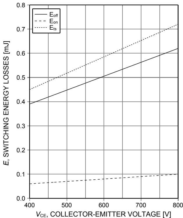
Figure 4. **Typical switching energy losses as a function of collector-emitter voltage**
