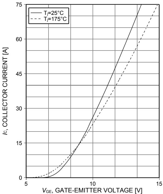
**Figure 7. Typical transfer characteristic**
