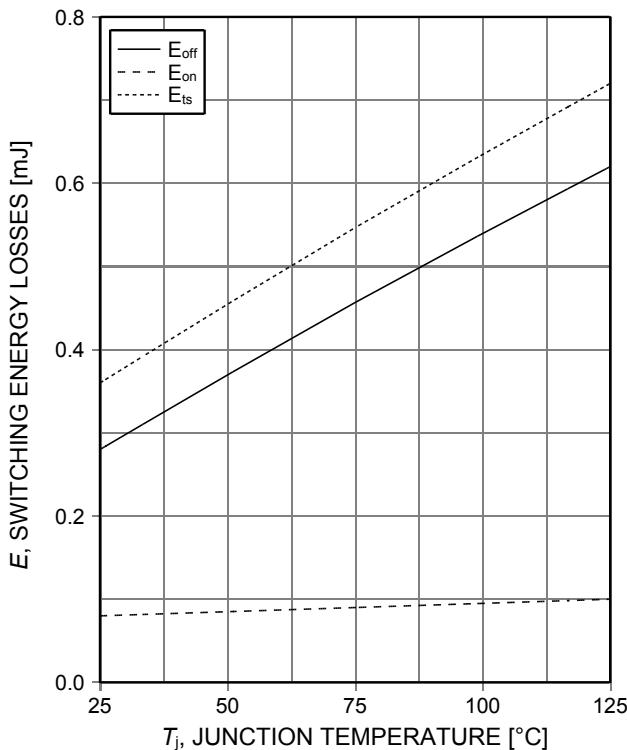
Figure 3. **Typical switching energy losses as a function of junction temperature**
