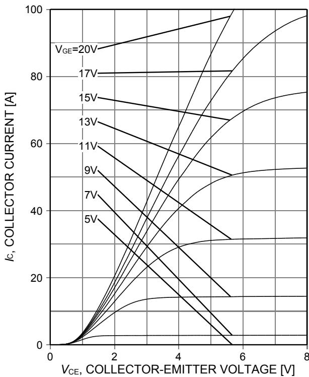
**Figure 6. Typical output characteristic**
