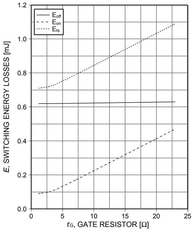
Figure 2. **Typical switching energy losses as a function of gate resistor**
