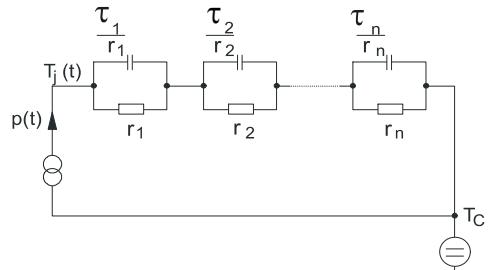
Figure D. Thermal equivalent circuit
