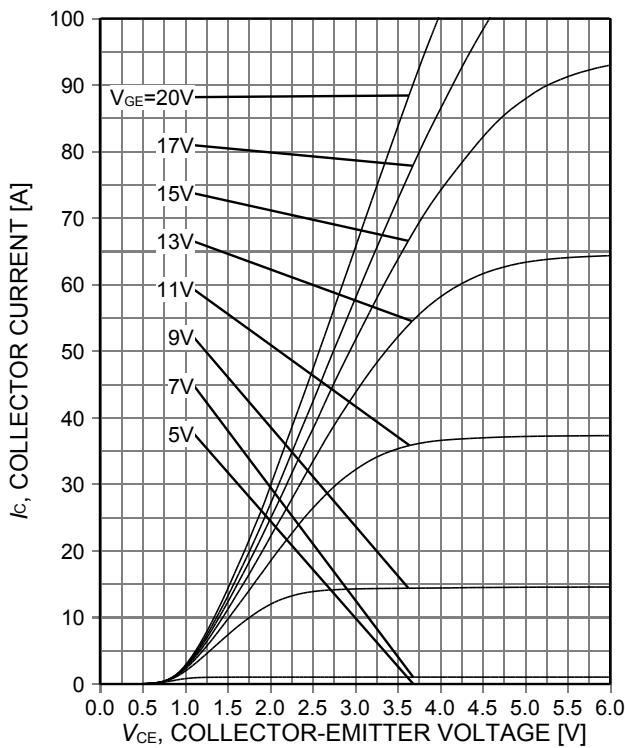
**Figure 5. Typical output characteristic**
