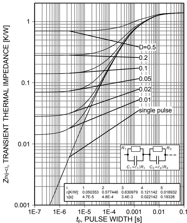
Figure 17. IGBT transient thermal impedance
