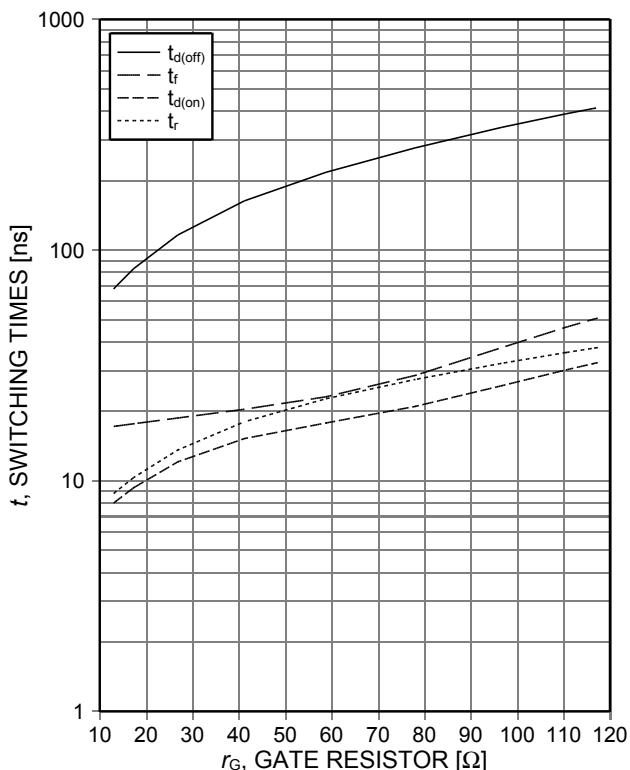
Figure 8. Typical switching times as a function of gate resistor
