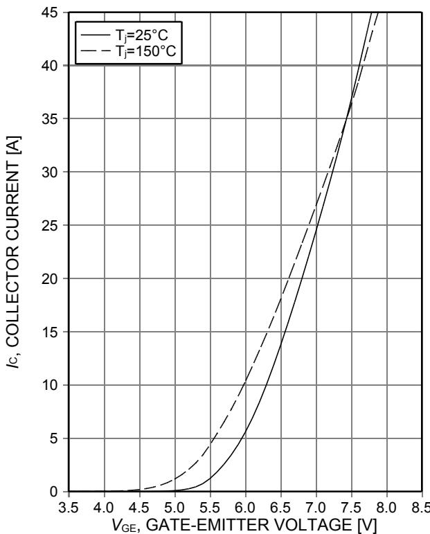
Figure 5. Typical transfer characteristic
