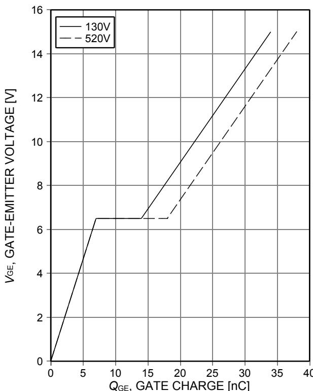
Figure 15. **Typical gate charge**
