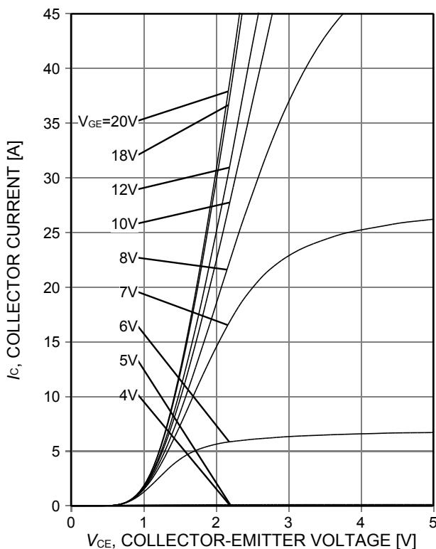
Figure 3. Typical output characteristic
