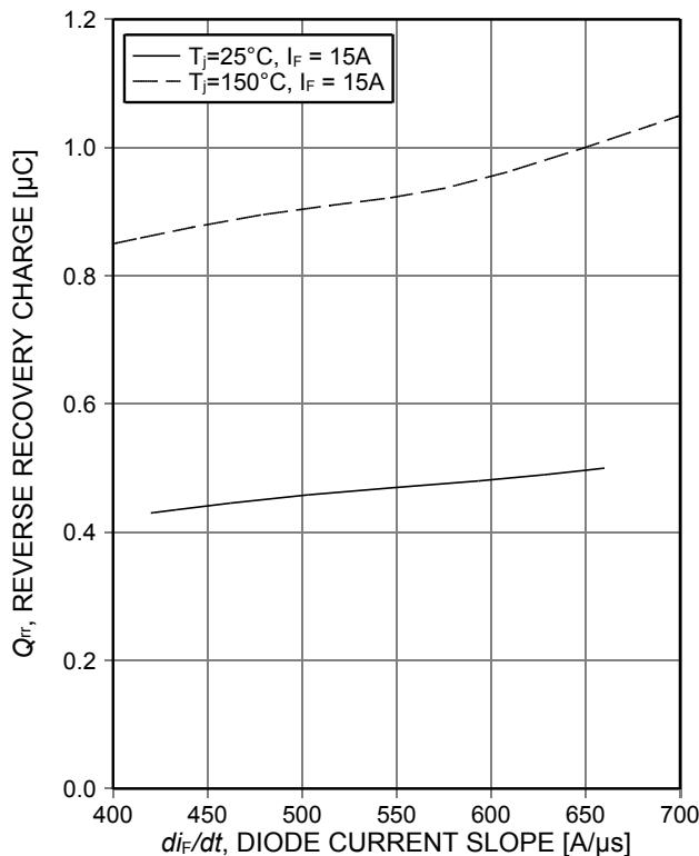
Figure 20. Typical reverse recovery charge as a function of diode current slope
