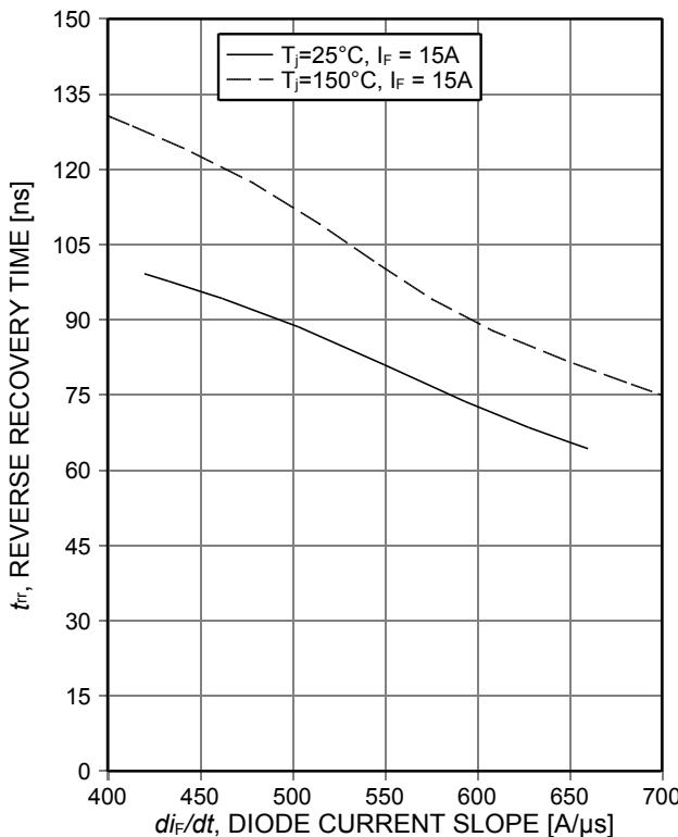
Figure 19. Typical reverse recovery time as a function of diode current slope
