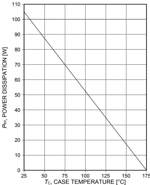
Figure 1. Power dissipation as a function of case temperature
