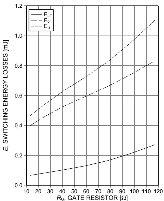
Figure 12. **Typical switching energy losses as a function of gate resistor**
