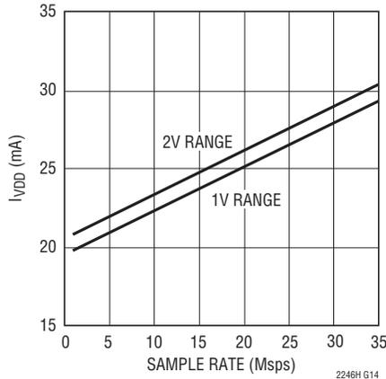
**$I_{QVDD}$  vs Sample Rate, 5MHz Sine
