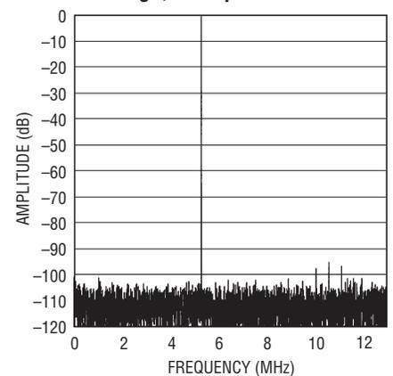
8192 Point FFT,  $f_{IN} = 30MHz$ ,  $-1dB$ , 2V Range, 25Mps
