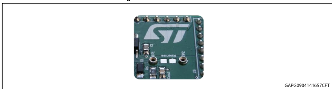
Figure 4: Mounting through-hole sense resistor
