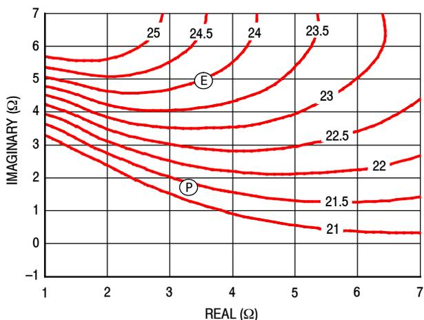
Figure 22. P1dB Load Pull Gain Contours (dB)
