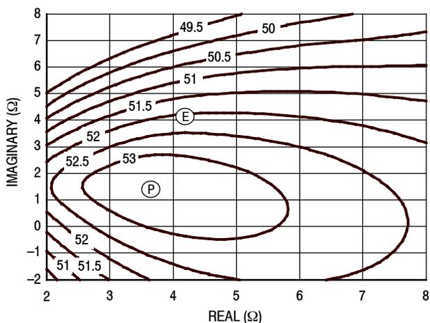
**Figure 24. P3dB Load Pull Output Power Contours (dBm)**
