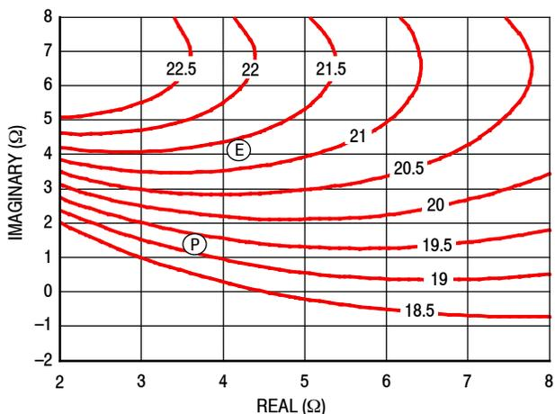
**Figure 26. P3dB Load Pull Gain Contours (dB)**
