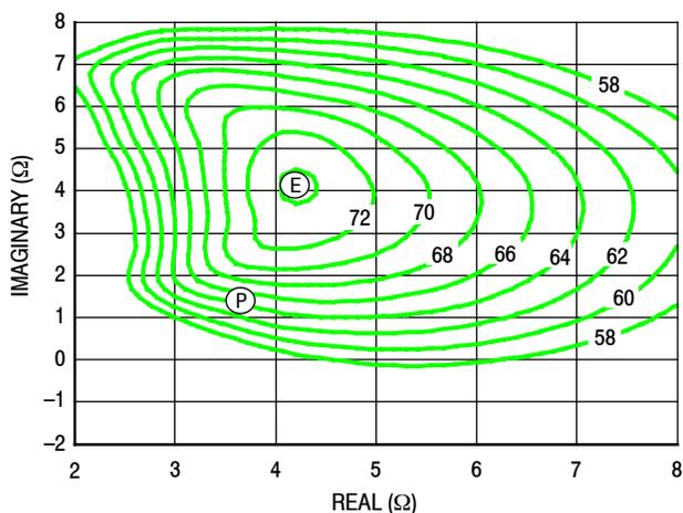
**Figure 25. P3dB Load Pull Efficiency Contours (%)**
