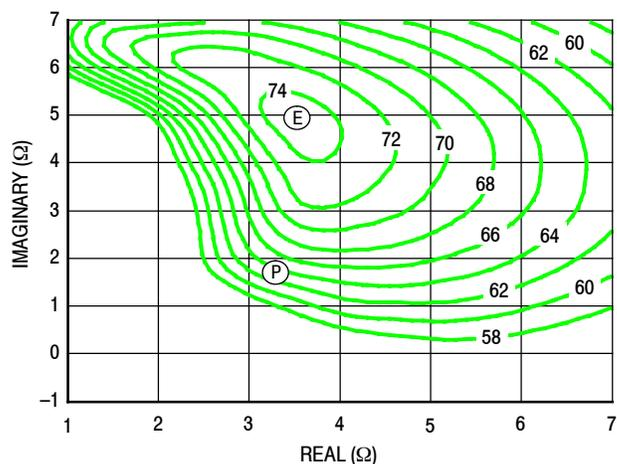
Figure 21. P1dB Load Pull Efficiency Contours (%)
