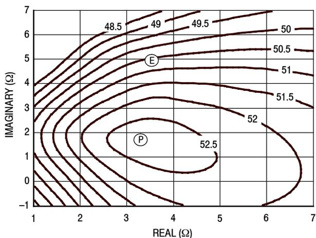
Figure 20. P1dB Load Pull Output Power Contours (dBm)
