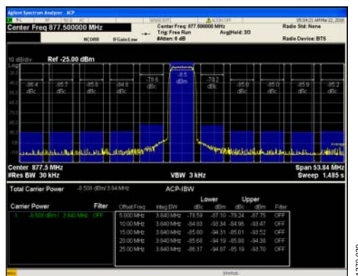
Figure 84. Single-Carrier W-CDMA at 877.5 MHz
