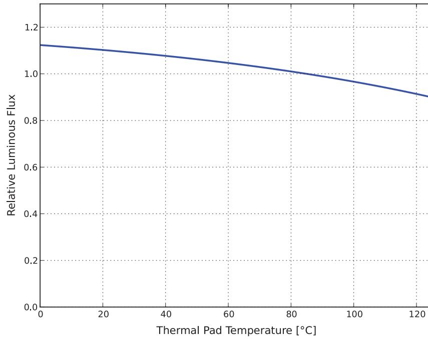
Figure 7. Relative light output vs. thermal pad temperature, LXAC-1827 and LXAC-1830.
