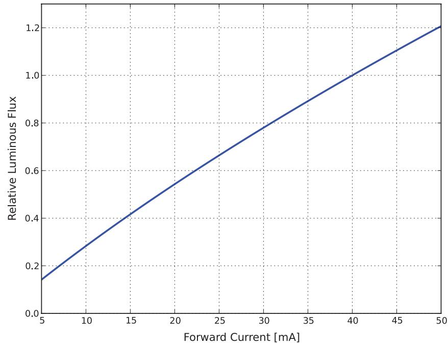
Figure 8. Typical relative luminous flux vs. forward current, LXAC-1827 and LXAC-1830.
