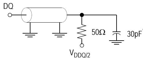
\* Distributed Test Jig Capacitance
