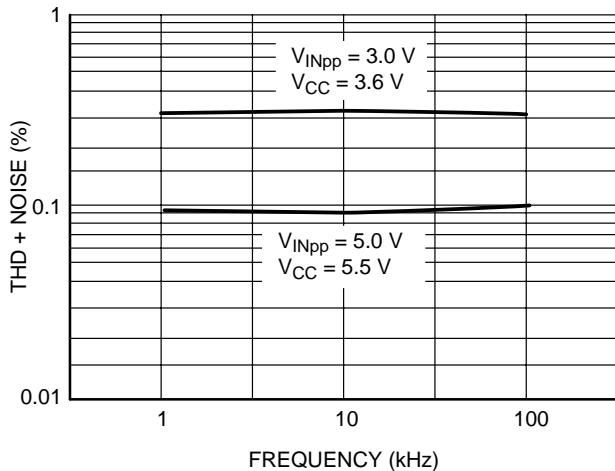
Figure 14. Total Harmonic Distortion Plus Noise vs. Frequency
