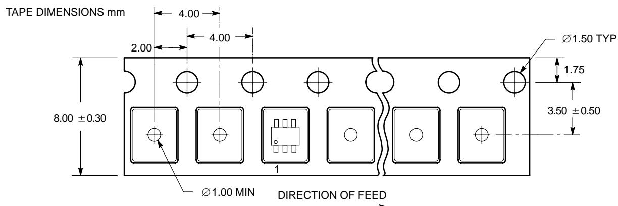
Figure 25. SC70-6/SC-88/SOT-363 DFT2 and SOT23-6/TSOP-6/SC59-6 DTT1 Reel Configuration/Orientation
