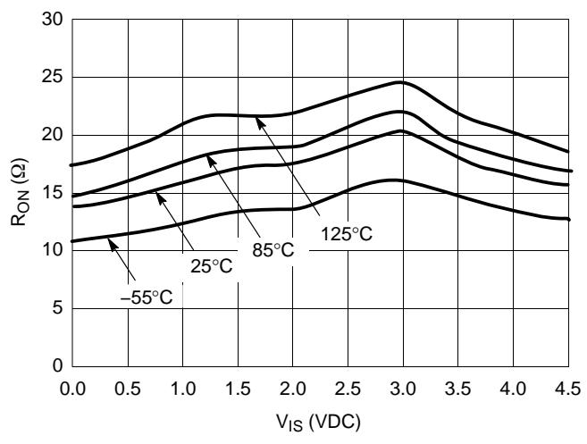
Figure 21.  $R_{ON}$  vs. Temp,  $V_{CC} = 4.5\text{ V}$
