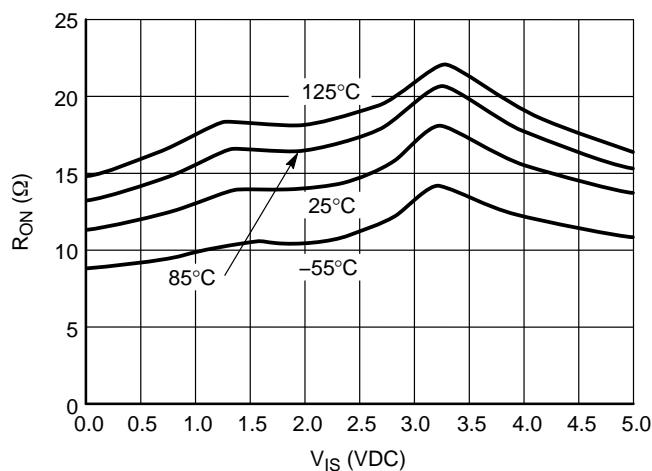
Figure 22. R<sub>ON</sub> vs. Temp, V<sub>CC</sub> = 5.0 V
