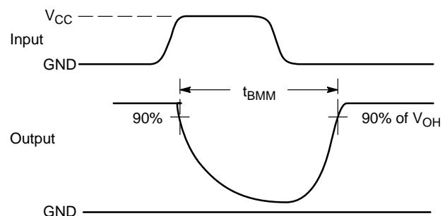
**Figure 4.  $t_{BBM}$  (Time Break-Before-Make)**
