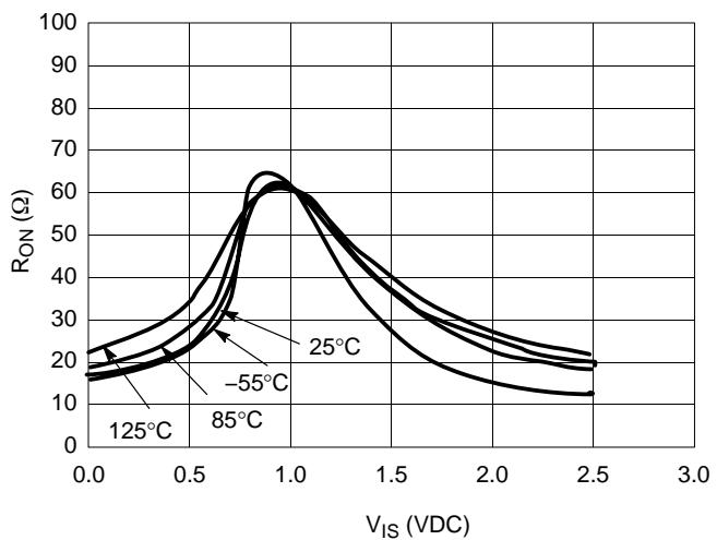
Figure 19.  $R_{ON}$  vs. Temp,  $V_{CC} = 2.5\text{ V}$
