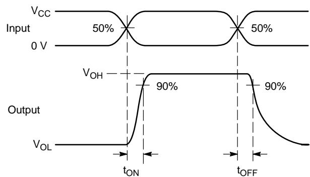
**Figure 5.  $t_{ON}/t_{OFF}$**
