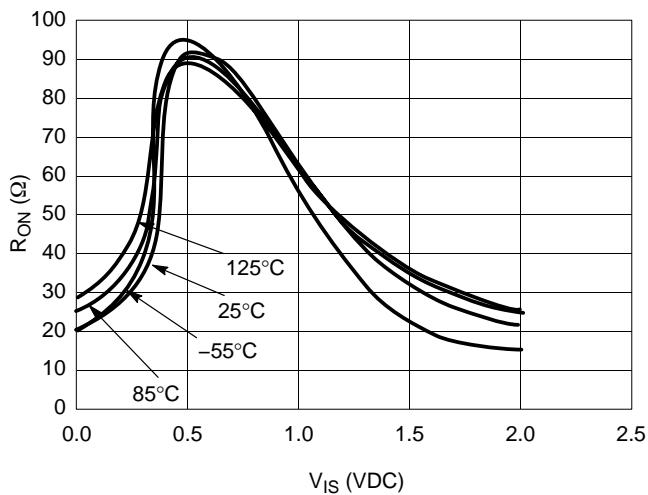
Figure 18.  $R_{ON}$  vs Temp,  $V_{CC} = 2.0\text{ V}$
