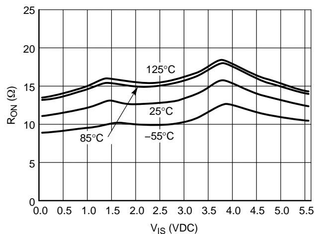
Figure 23. R<sub>ON</sub> vs. Temp, V<sub>CC</sub> = 5.5 V
