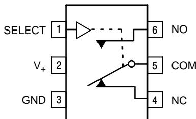
Figure 1. Pin Assignment
