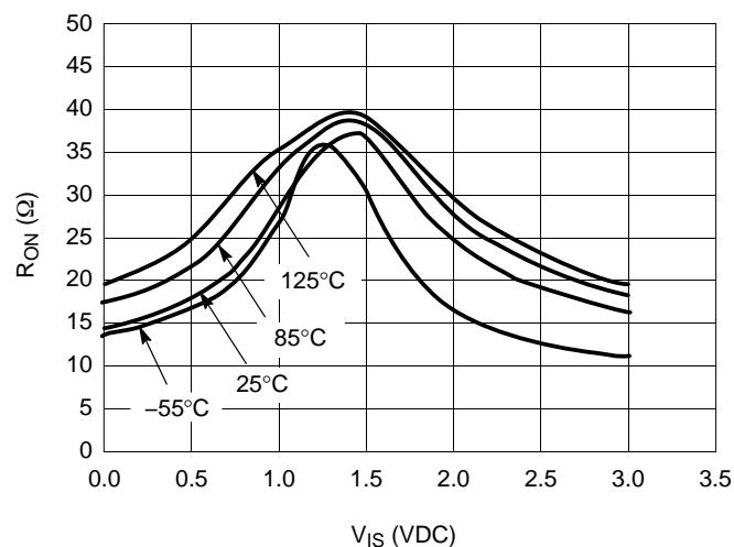
Figure 20.  $R_{ON}$  vs. Temp,  $V_{CC} = 3.0\text{ V}$
