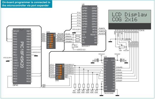
Figure 20-2: On-board 2x16 LCD and microcontroller connection schematic
