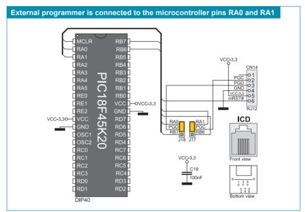
Figure 5-2: ICD connector and microcontroller connection schematic
