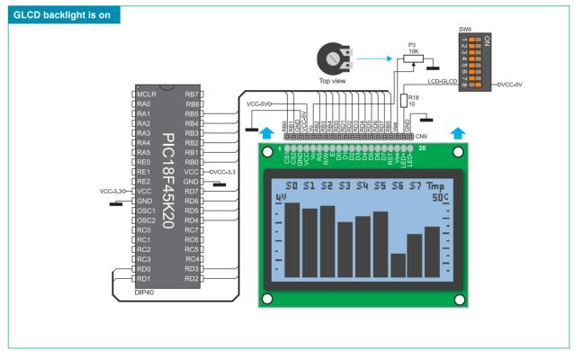
Figure 22-3: GLCD and microcontroller connection schematic
