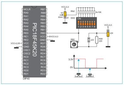
In order to enable port PORTB pins to be connected to pull-up resistors and the port input pins to be supplied with a logic zero (0), it is necessary to place jumper J2 in the *Up* position and jumper J23 in the GND position. This enables any port PORTB input pin to be driven high (3.3V) in idle state over the 10k resistor.
