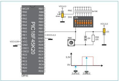
In order to enable the PORTB port pins to be connected to pull-down resistors, it is necessary to place jumper J2 in the *Down* position first. This enables any PORTB port pin to be supplied with a logic zero (0V) in idle state over jumper J2 and 8x10k resistor network. To provide the RB0 pin with such signal, it is necessary to set switch 1 on the DIP switch SW2 to ON position.
