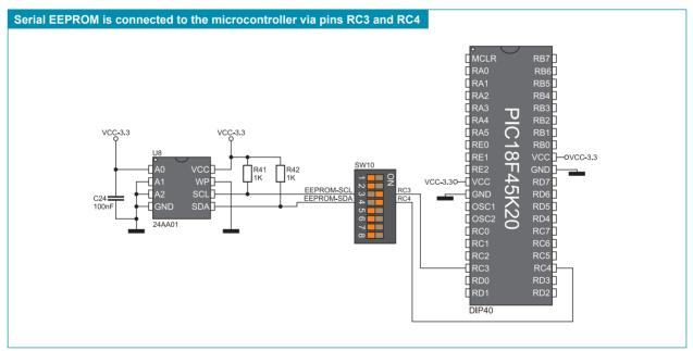
Figure 12-2: Serial EEPROM module and microcontroller connection schematic
