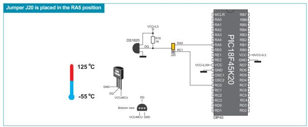
Figure 14-4: DS1820 temperature sensor and microcontroller connection schematic
