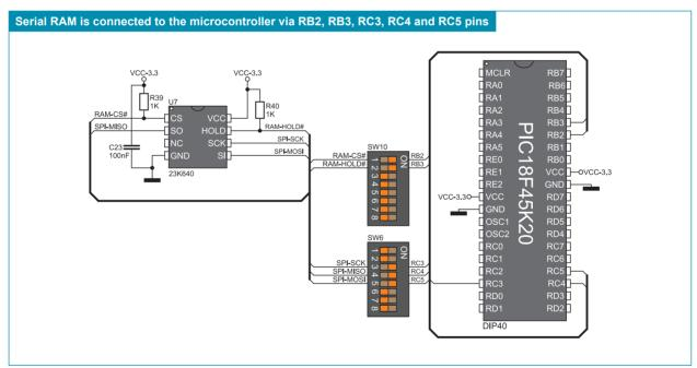
Figure 13-2: Serial RAM module and microcontroller connection schematic
