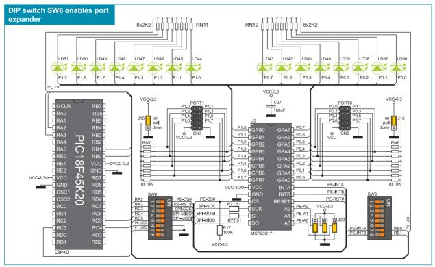
Figure 25-2: Port expander and microcontroller connection schematic
