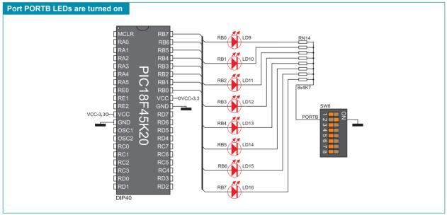
Figure 16-2: LEDs and port PORTB connection schematic
