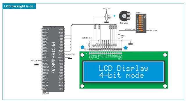
Figure 21-3: Alphanumeric 2x16 LCD and microcontroller connection schematic
