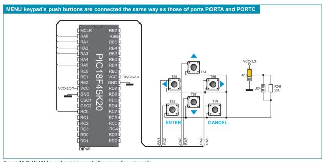
Figure 18-2: MENU keypad and microcontroller connection schematic
