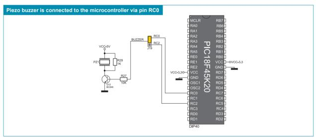
Figure 15-4: Piezo buzzer and microcontroller connection schematic
