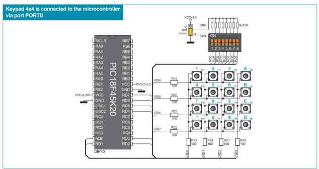
Figure 17-3: Keypad 4x4 and microcontroller connection schematic
