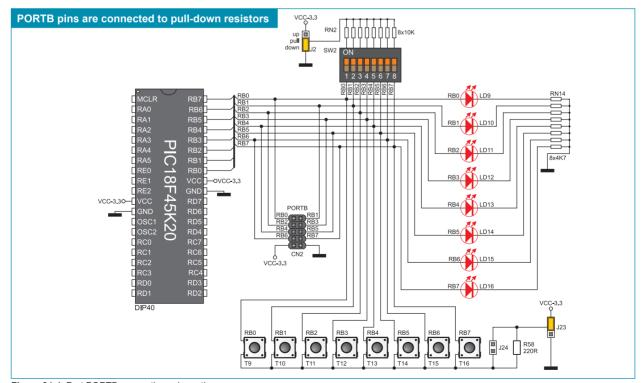
Figure 24-4: Port PORTB connection schematic
