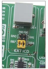
Figure 5-1: ICD connector
