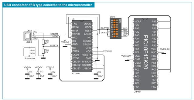
Figure 10-2: USB connector and microcontroller connection schematic
