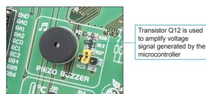
Figure 15-1: Piezo buzzer
