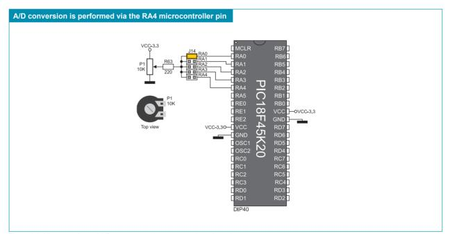
Figure 9-3: Microcontroller and A/D converter test inputs connection schematic
