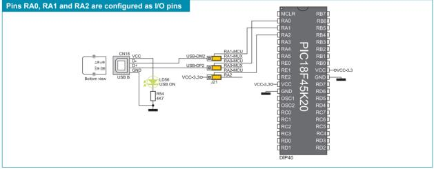
Figure 8-3: CN18 USB connector and microcontroller schematic
