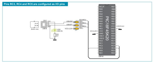
Figure 8-2: CN11 USB connector and microcontroller schematic
