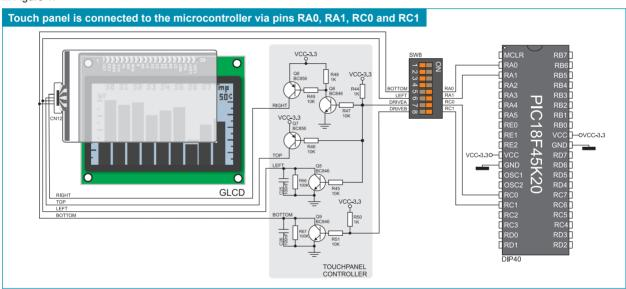
Figure 23-2: Touch panel and microcontroller connection schematic
