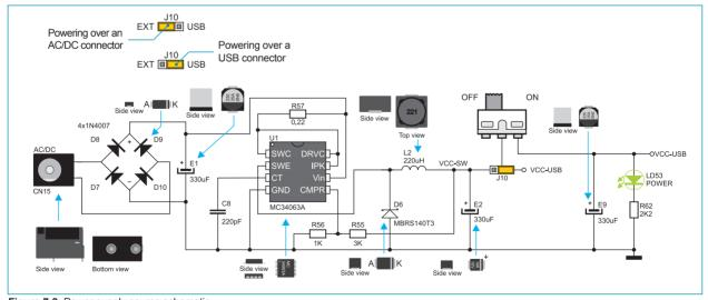
Figure 7-2: Power supply source schematic
