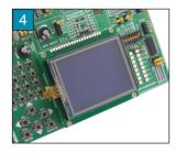
Figure 23-1: Placing touch panel over a GLCD
