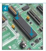
Figure 2-2: Plugging microcontroller into appropriate socket
