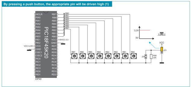
Figure 19-2: Push buttons and port PORTB connection schematic
