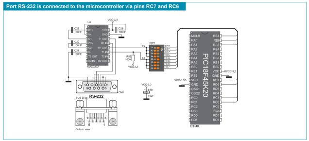
Figure 11-2: RS-232 module ad microcontroller connection schematic
