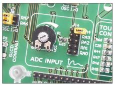
Figure 9-1: ADC (jumper's default position)
