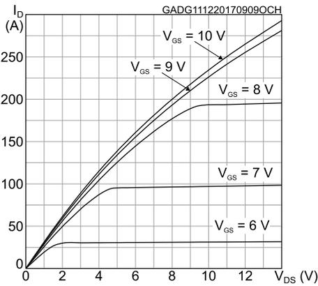
Figure 4. Transfer characteristics
