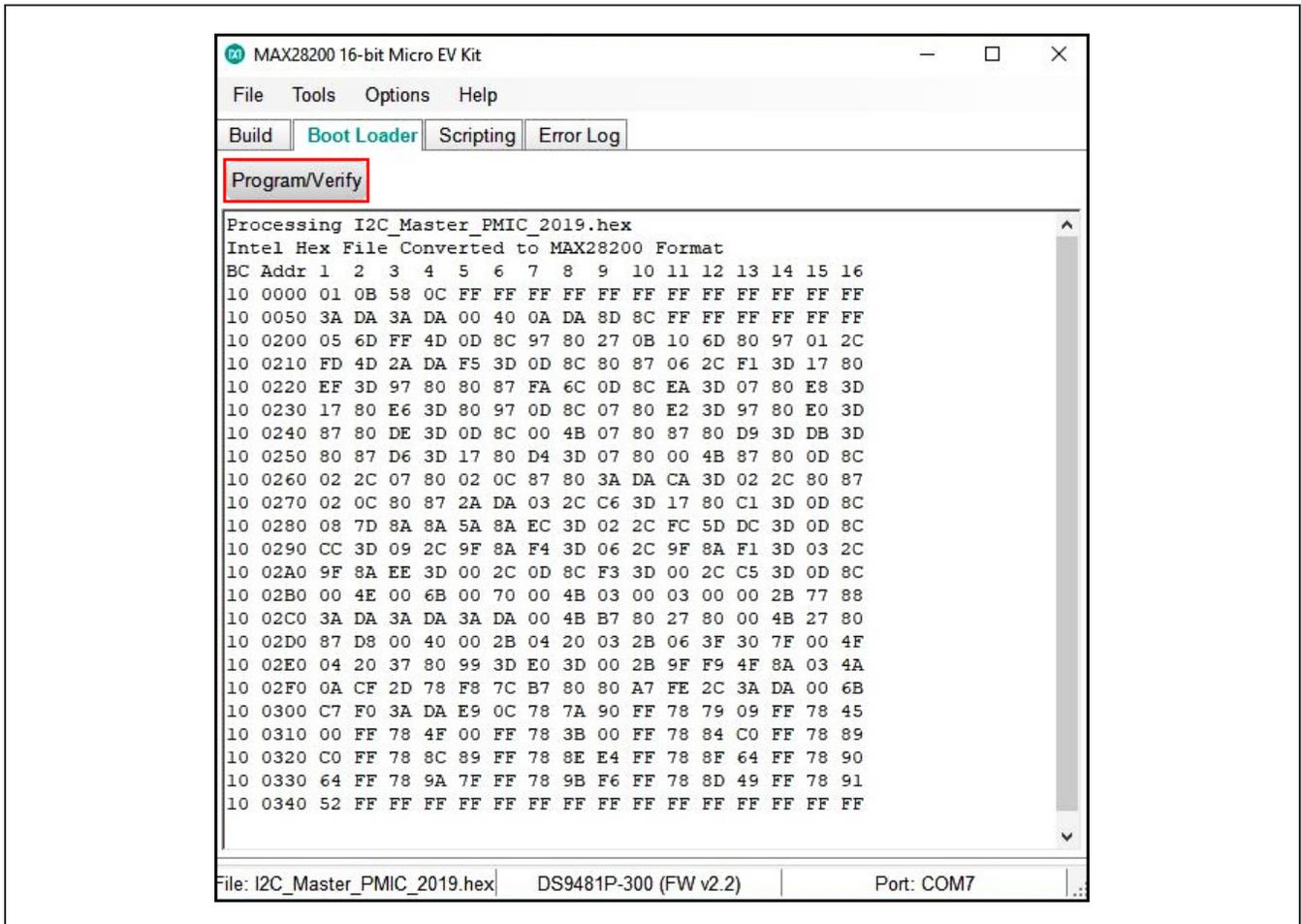
Figure 16. Program the Device with the Data Pattern
