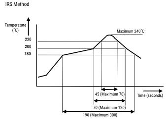
Note: Temperature profile shows printed circuit board surface temperature on the relay terminal portion. Please consult KEMET if you wish to use a temperature profile other than above.
