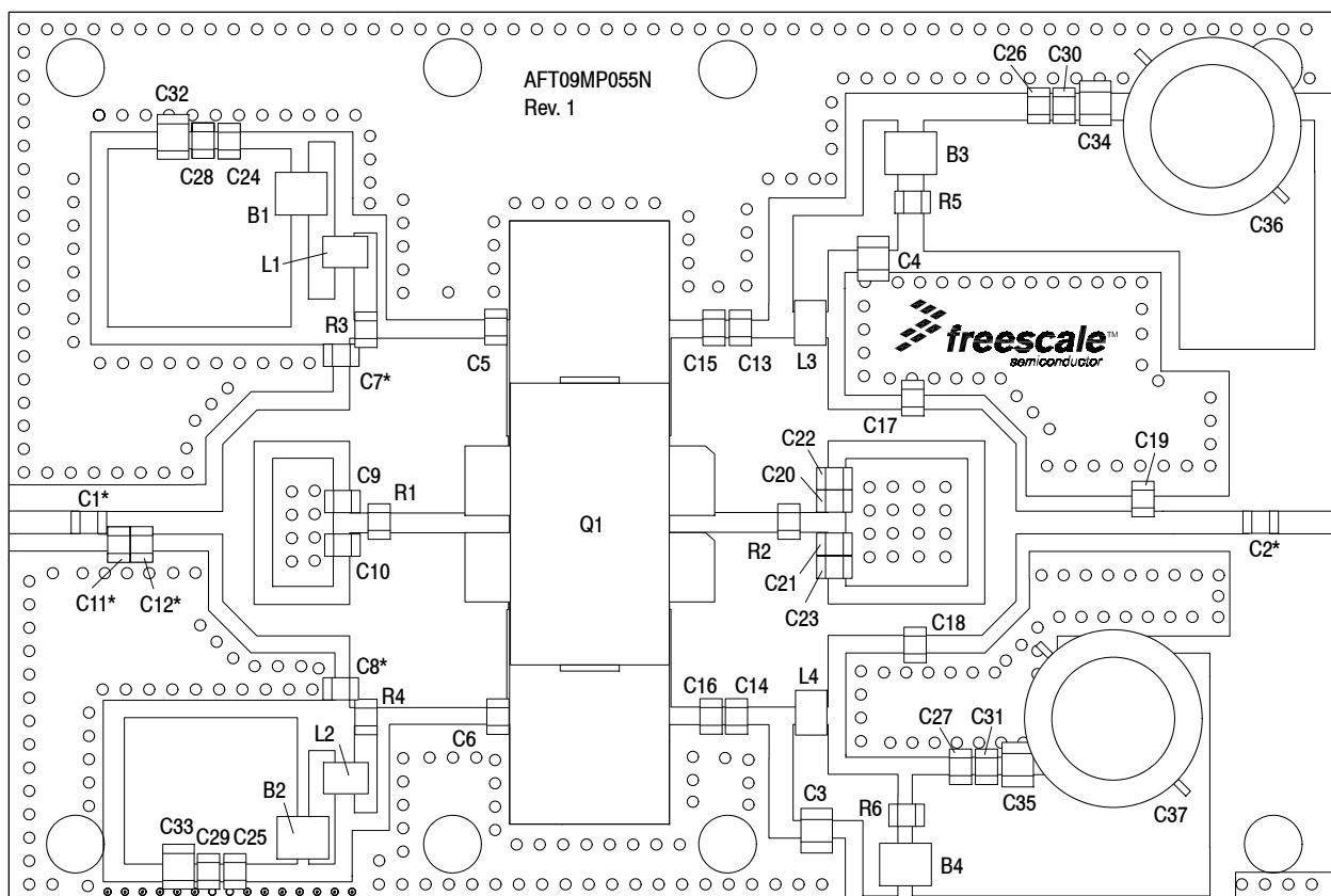
\*C1, C2, C7, C8, C11 and C12 are mounted vertically.
