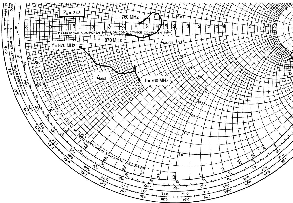
$V_{DD} = 12.5 \text{ Vdc}$ ,  $I_{DQ(A+B)} = 800 \text{ mA}$ ,  $P_{out} = 55 \text{ W Avg.}$
