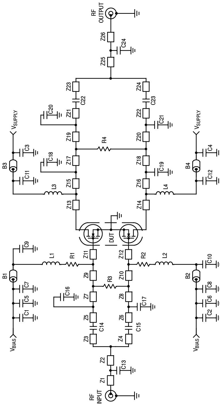
**Figure 6. AFT09MP055NR1 Narrowband Test Circuit Schematic — 870 MHz**
