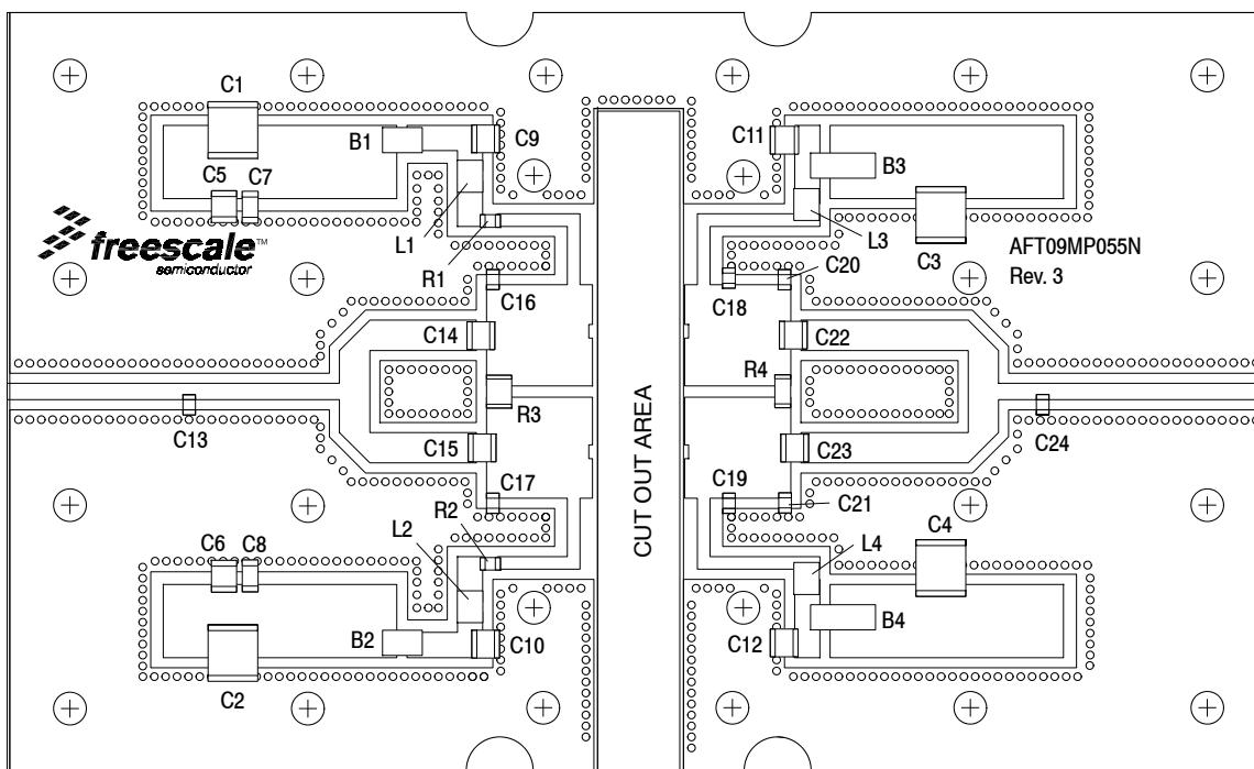
Figure 5. AFT09MP055NR1 Narrowband Test Circuit Component Layout — 870 MHz
