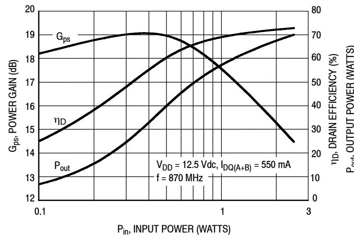
Figure 8. Power Gain, Drain Efficiency and Output
