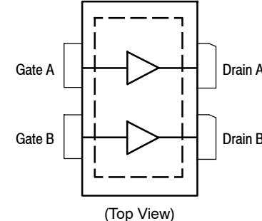
Note: Exposed backside of the package is the source terminal for the transistor.
