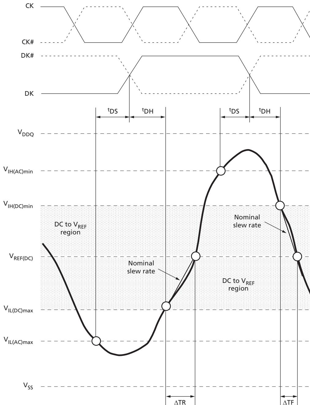
$$\text{Hold slew rate}_{\text{rising signal}} = \frac{V_{REF(DC)} - V_{IL(DC)max}}{\Delta TR}$$
