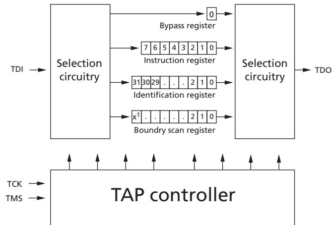
Note: 1.  $x = \text{Die Rev. A} = 121$  for all configurations, Die Rev. B = 135 for all configurations.
