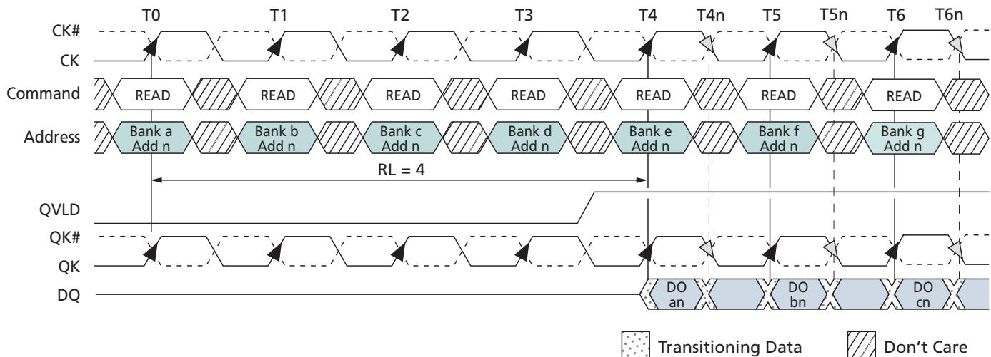
Note: 1. DO an (or bn, cn) = data-out from bank a (or bank b, c) and address n.
