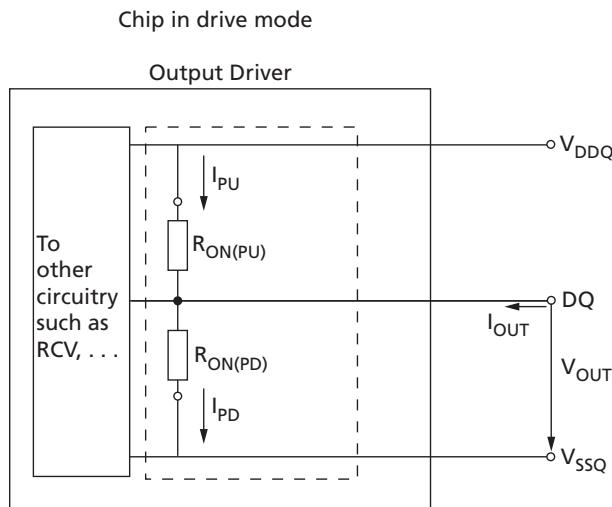
**Table 20: Driver Pull-Up and Pull-Down Impedance Calculations**
