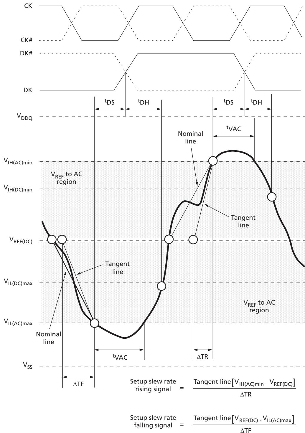
Note: 1. Both the clock and the strobe are drawn on different time scales.
