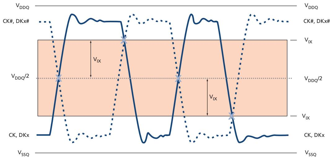
**Figure 10: Single-Ended Requirements for Differential Signals**
