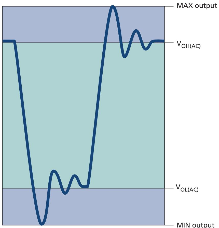
**Figure 17: Differential Output Signal**
