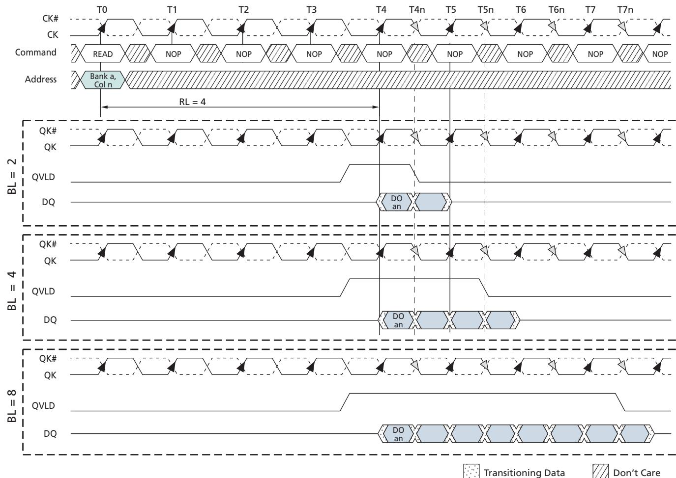
Note: 1. DO an = data-out from bank a and address an.
