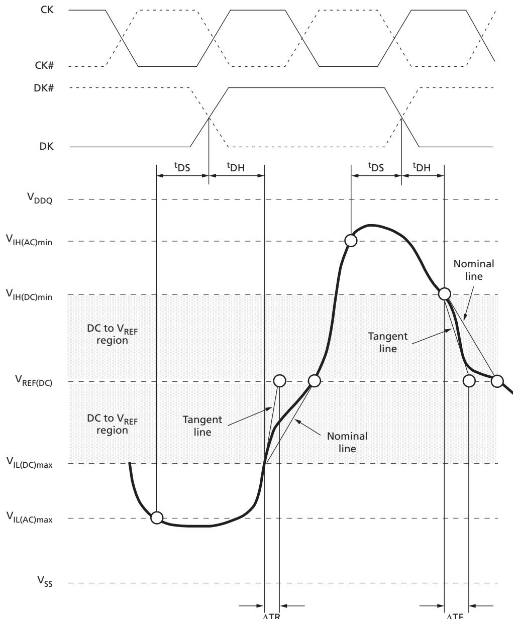
$$\text{Hold slew rate rising signal} = \frac{\text{Tangent line} [V_{REF(DC)} - V_{IL(DC)\text{max}}]}{\Delta TR}$$
