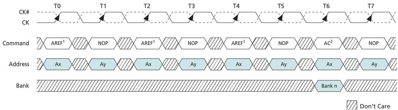
Notes: 1. Usage of multibank AREF subject to  $t_{SAW}$  and  $t_{MMD}$  specifications.
