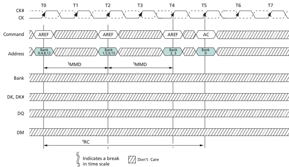
**Figure 55: READ Burst with ODT**
