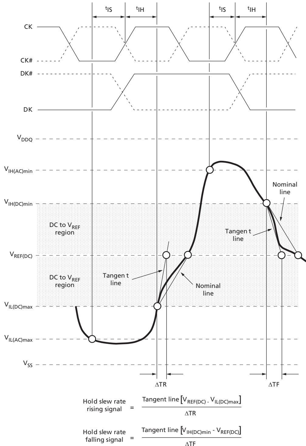
Note: 1. Both the clock and the data strobe are drawn on different time scales.
