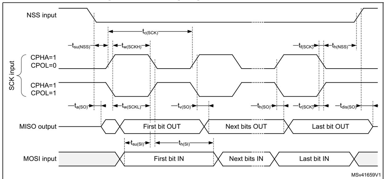
Figure 36. SPI timing diagram - master mode<sup>(1)</sup>
