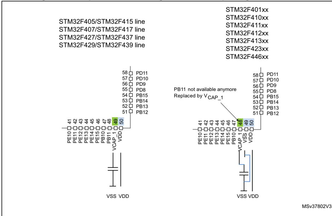
Figure 2. Compatible board design for LQFP64 package
