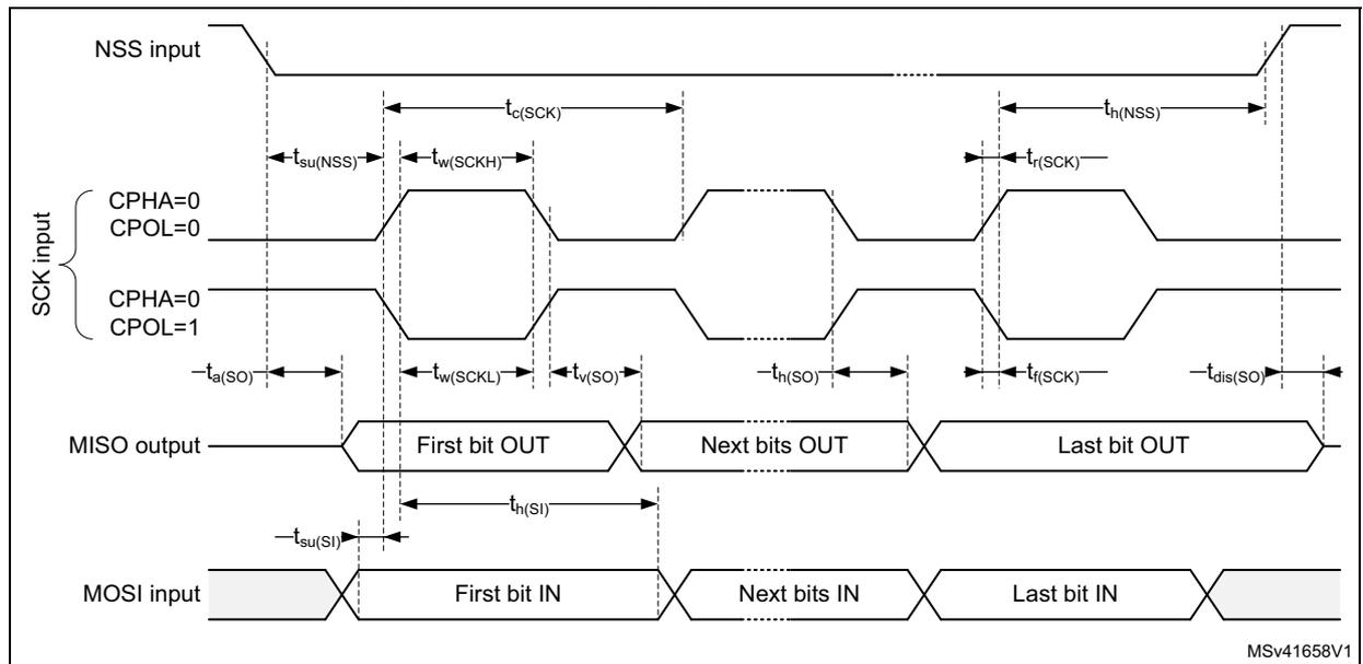
Figure 35. SPI timing diagram - slave mode and CPHA = 1<sup>(1)</sup>
