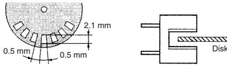
3. The following illustrations show the definition of response delay time. The value in the parentheses applies to the EE-SX4088.
