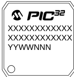
100-Lead TQFP (12x12x1 mm)
