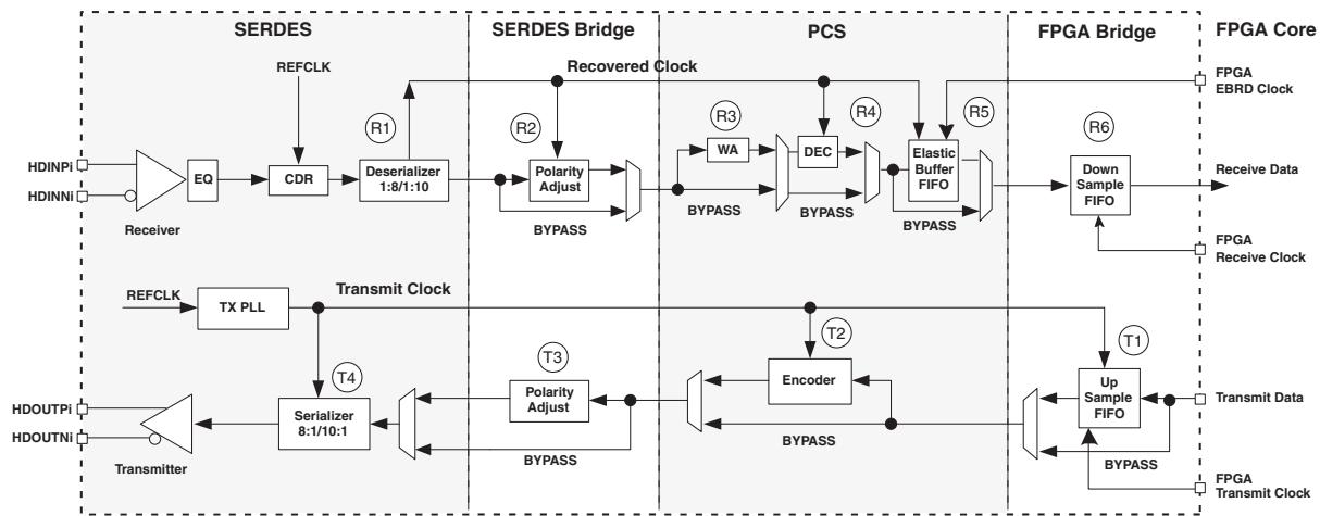
**SERDES High Speed Data Receiver (LatticeECP2M Family Only)****Table 3-11. Serial Input Data Specifications**
