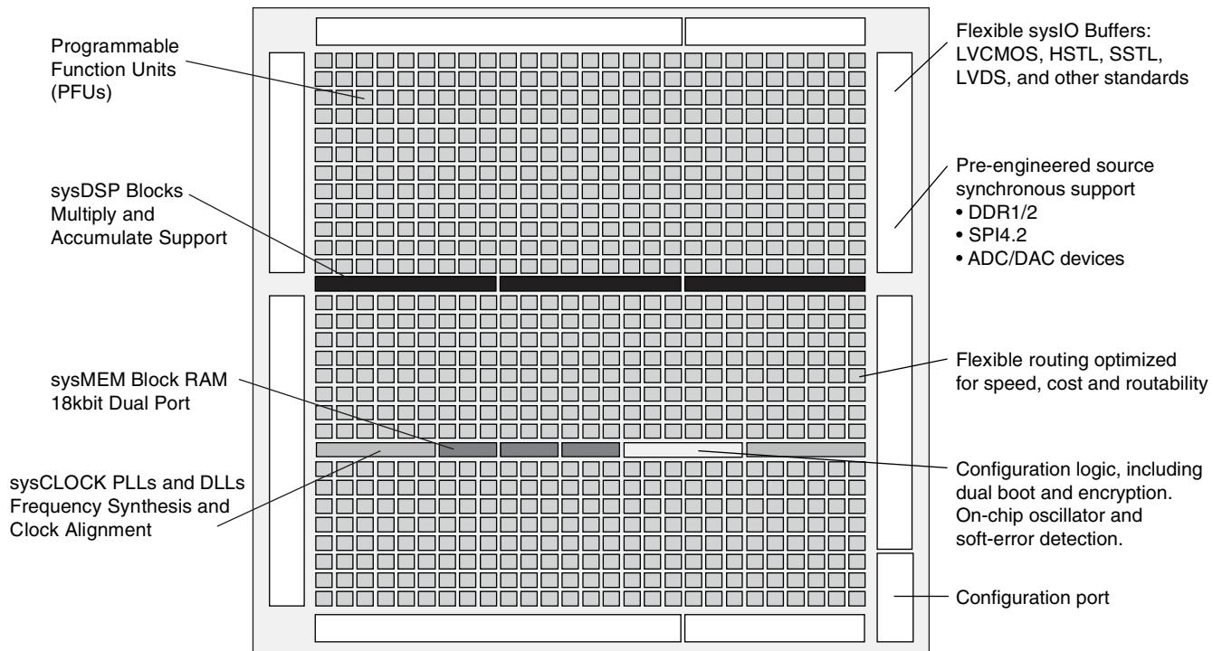
**Figure 2-2. Simplified Block Diagram, ECP2M20 Device (Top Level)**
