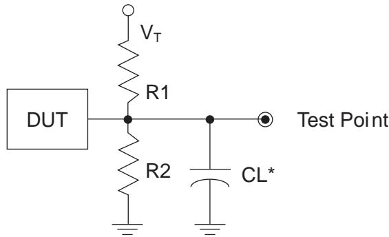
\*CL Includes Test Fixture and Probe Capacitance
