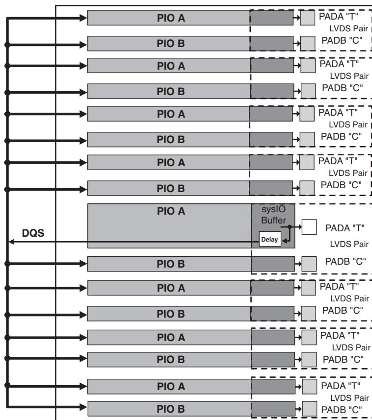
**Figure 2-34. DQS Input Routing for the Bottom Edge of the Device**
