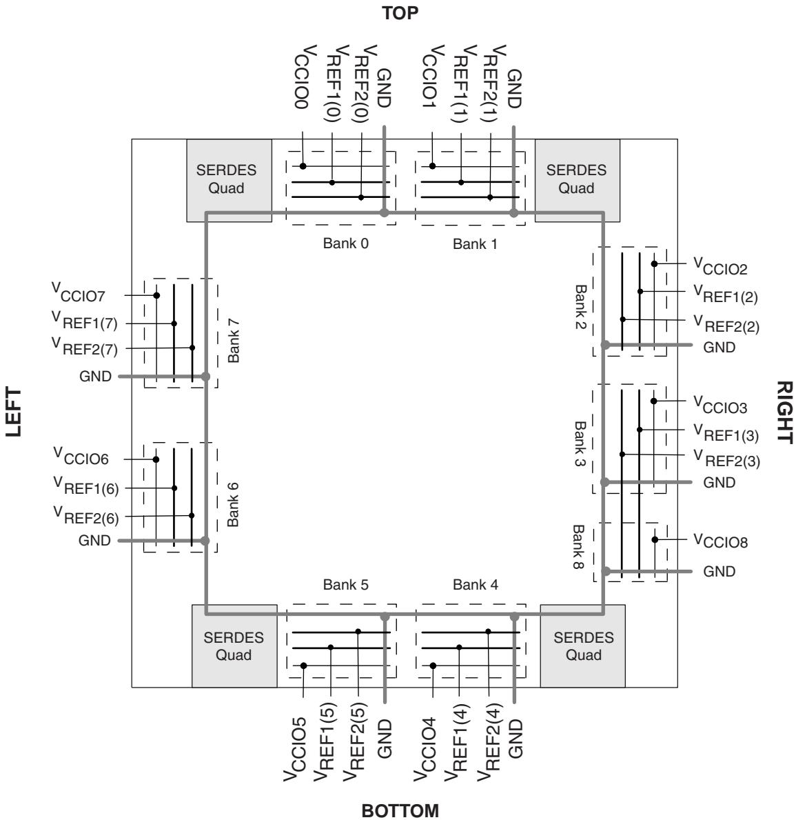
LatticeECP2/M devices contain two types of sysl/O buffer pairs.
