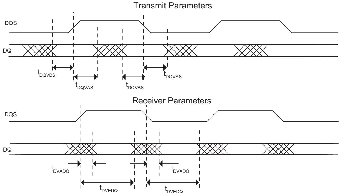
**Figure 3-8. XGMII Parameters**
