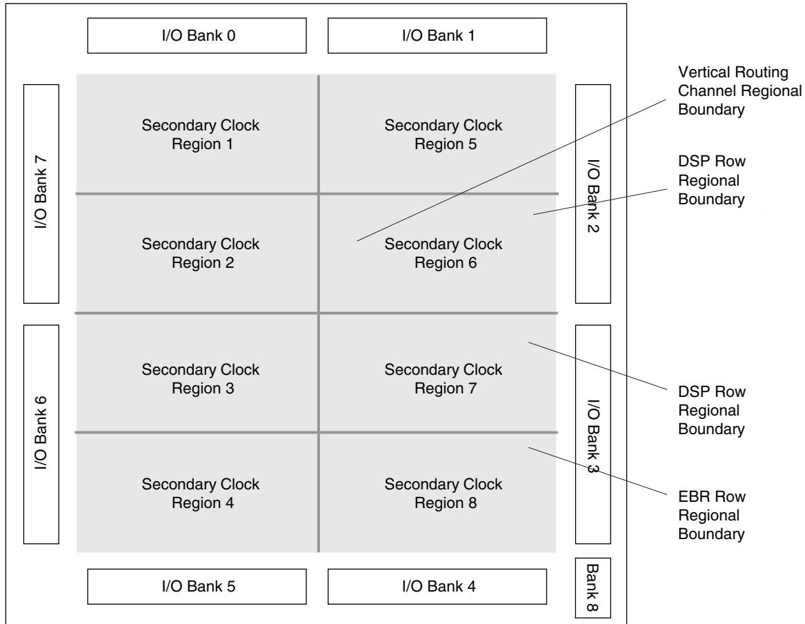
**Figure 2-16. Secondary Clock Selection**
