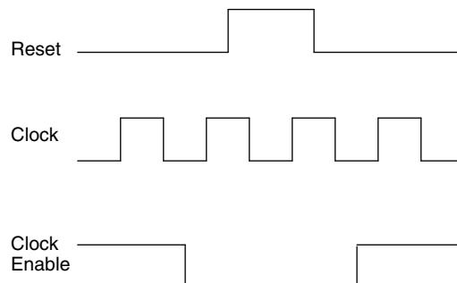
If all clock enables remain enabled, the EBR asynchronous reset or GSR may only be applied and released after the EBR read and write clock inputs are in a steady state condition for a minimum of  $1/f_{MAX}$  (EBR clock). The reset release must adhere to the EBR synchronous reset setup time before the next active read or write clock edge.
