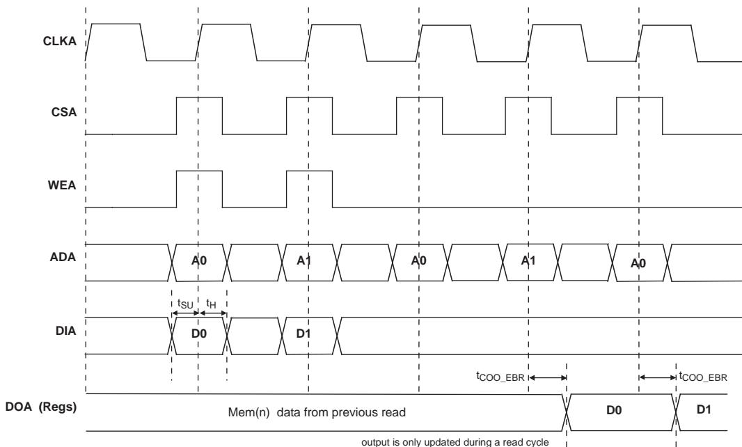
**Figure 3-11. Write Through (SP Read/Write on Port A, Input Registers Only)**
