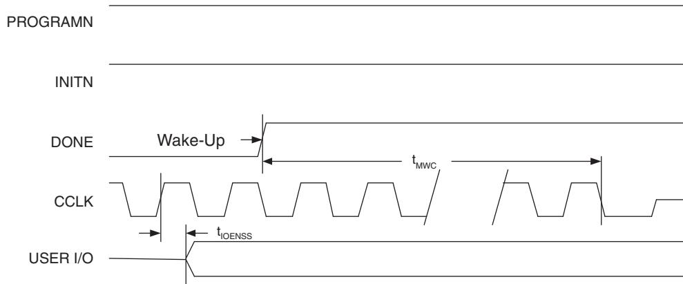
**Figure 3-20. SPI/SPI<sub>M</sub> Configuration Waveforms**
