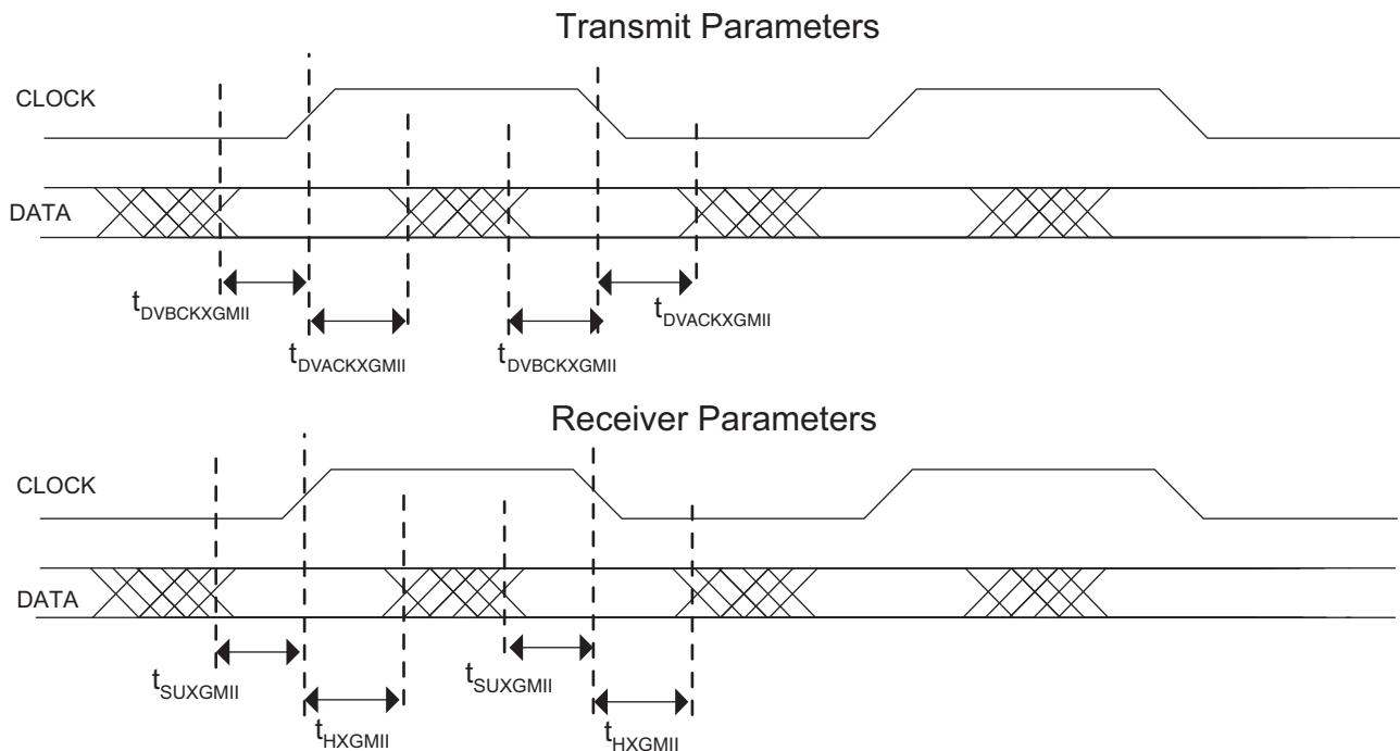
**LatticeECP2/M Internal Switching Characteristics<sup>1</sup>**
