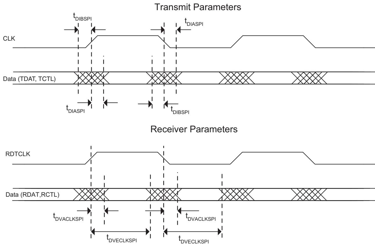
**Figure 3-7. DDR and DDR2 Parameters**
