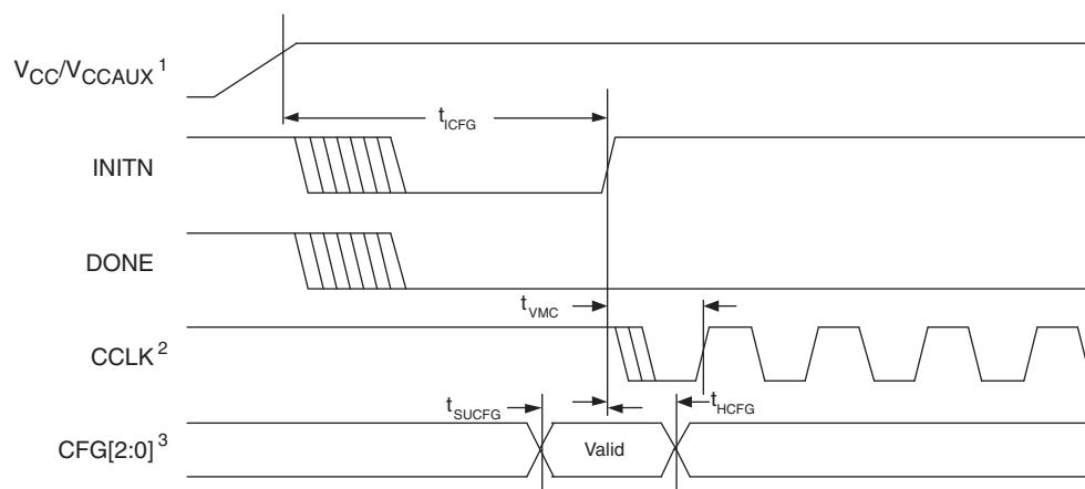
1. Time taken from  $V_{CC}$  or  $V_{CCAUX}$ , whichever is the last to reach its  $V_{MIN}$ .
