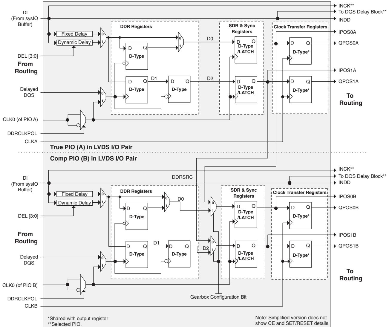
**Figure 2-30. Input Register Block Top Edge**
