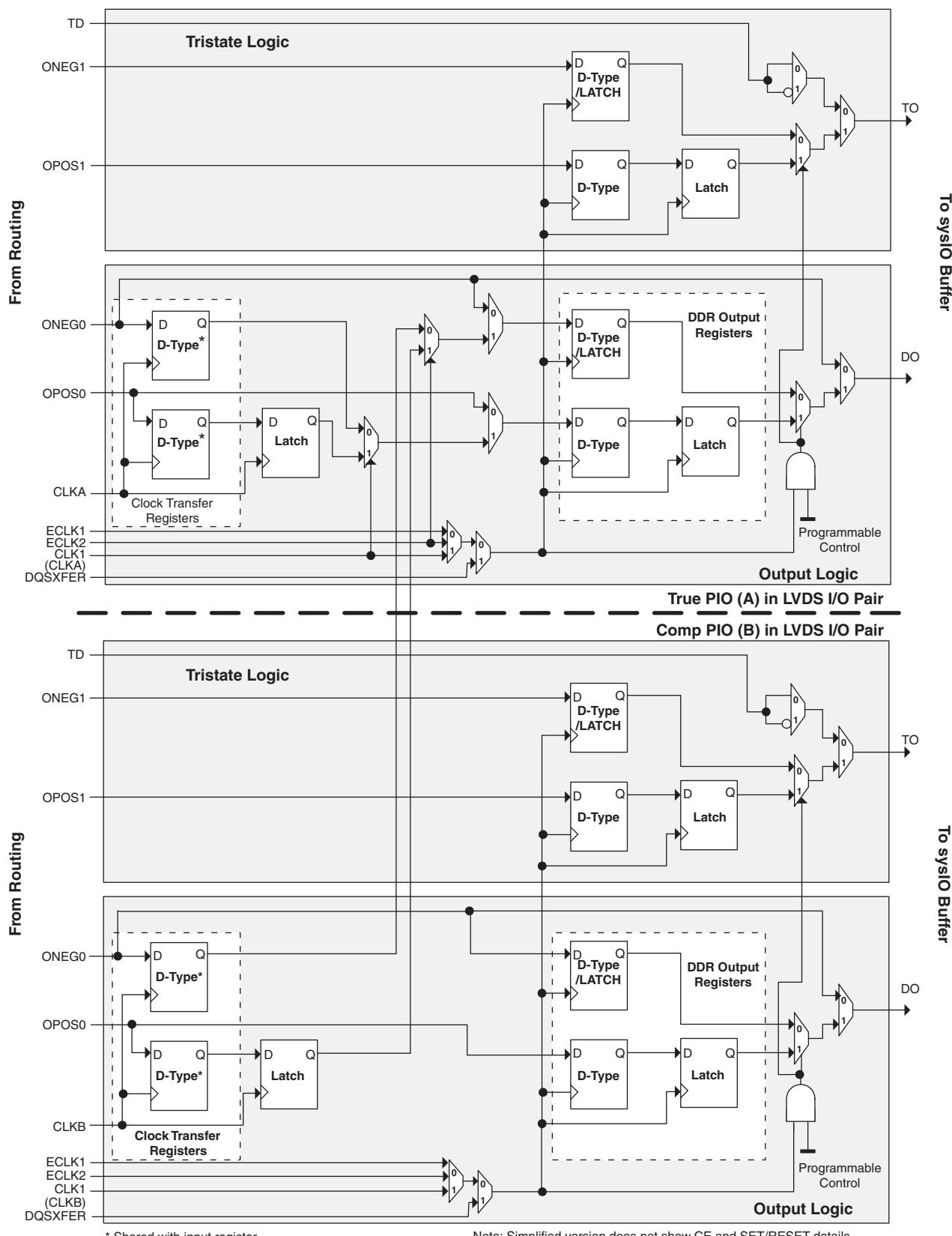
**Figure 2-32. Output and Tristate Block, Top Edge**
