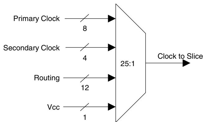
**Figure 2-18. Slice0 through Slice2 Control Selection**
