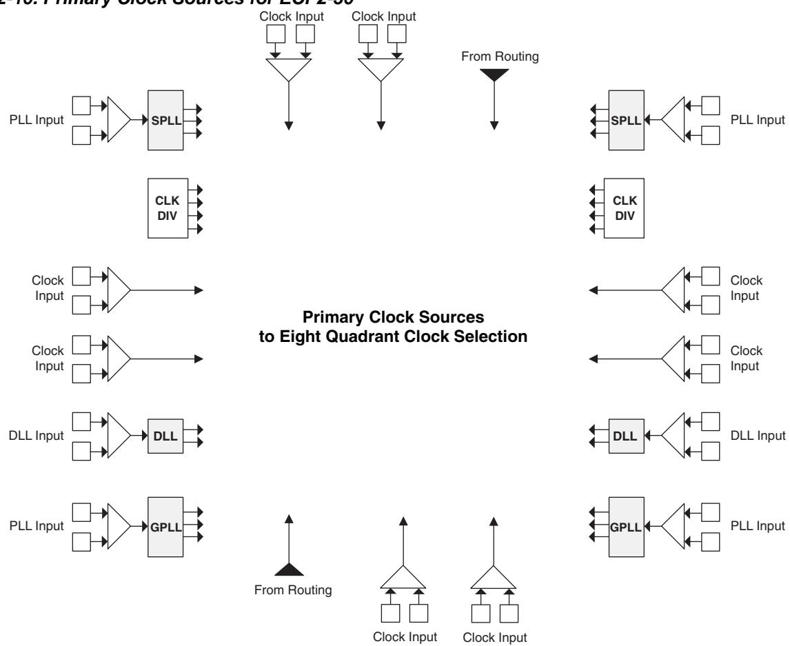
Note: This diagram shows sources for the ECP2-50 device. Smaller LatticeECP2 devices have fewer SPLLs. All LatticeECP2M device have six SPLLs.
