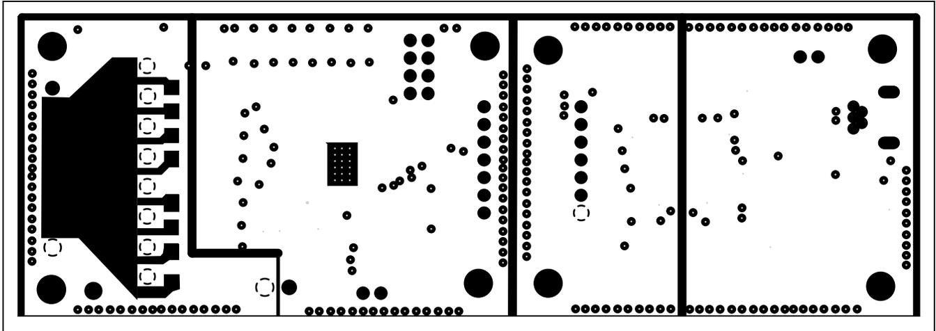
Figure 6. MAX31912/MAX31913 EV Kit PCB Layout—Internal Layer 2
