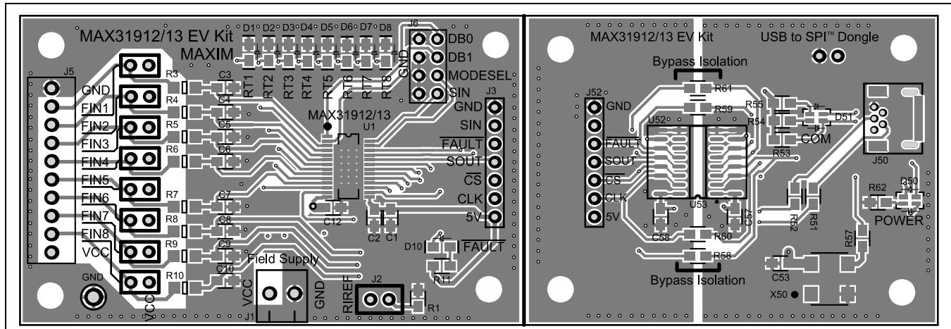
Figure 4. MAX31912/MAX31913 EV Kit PCB Layout—Top
