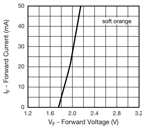
Fig. 3 - Forward Current vs. Forward Voltage (soft orange)
