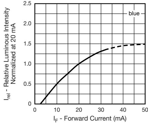
Fig. 15 - Relative Luminous Intensity vs. Forward Current (blue)
