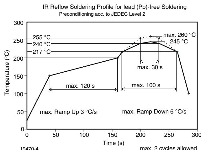
Fig. 19 - Vishay Lead (Pb)-free Reflow Soldering Profile
