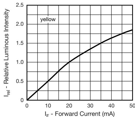
Fig. 8 - Relative Luminous Intensity vs. Forward Current (yellow)
