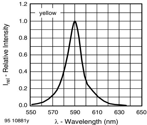
Fig. 12 - Relative Intensity vs. Wavelength (yellow)
