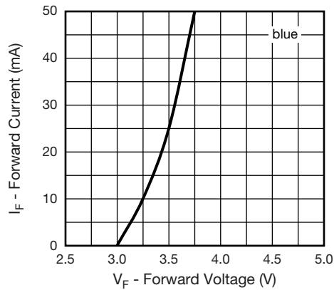
Fig. 14 - Forward Current vs. Forward Voltage (blue)
