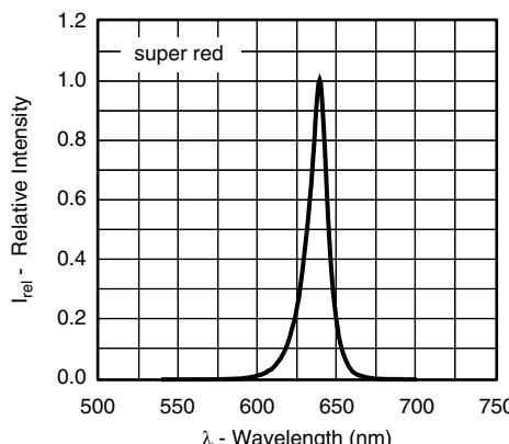
Fig. 10 - Relative Intensity vs. Wavelength (super red)
