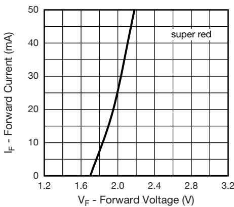
Fig. 2 - Forward Current vs. Forward Voltage (super red)
