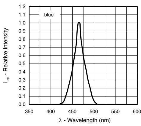
Fig. 16 - Relative Intensity vs. Wavelength (blue)
