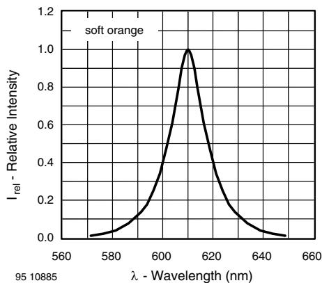
Fig. 11 - Relative Intensity vs. Wavelength (soft orange)
