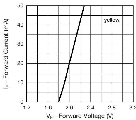
Fig. 4 - Forward Current vs. Forward Voltage (yellow)
