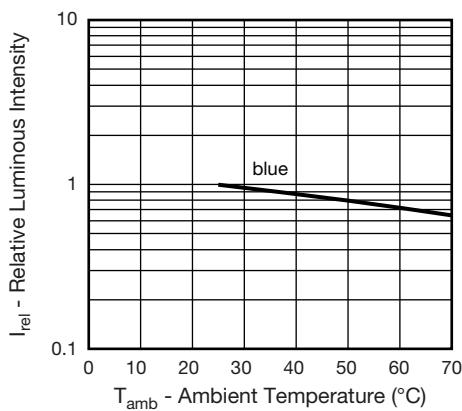
Fig. 17 - Relative Luminous Intensity vs. Ambient Temperature
