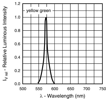
Fig. 13 - Relative Intensity vs. Wavelength (yellow green)
