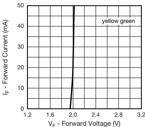
Fig. 5 - Forward Current vs. Forward Voltage (yellow green)
