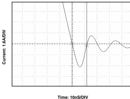
**Figure 23.** FDS6900AS SyncFET body diode reverse recovery characteristic.
