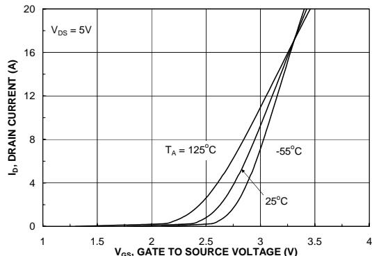
**Figure 16. Transfer Characteristics.**
