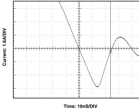
**Figure 24.** Non-SyncFET (FDS6690) body diode reverse recovery characteristic.
