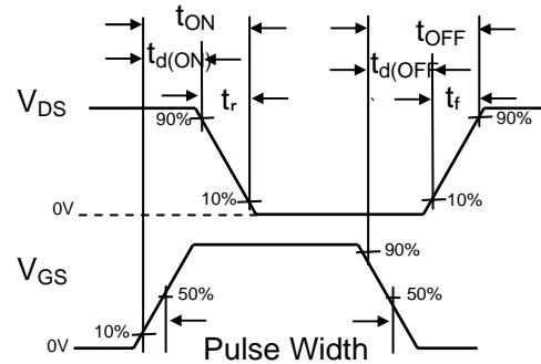
Figure 31. Switching Time Waveforms
