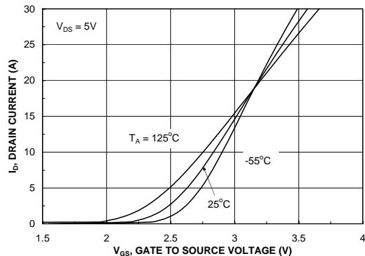
**Figure 5. Transfer Characteristics.**
