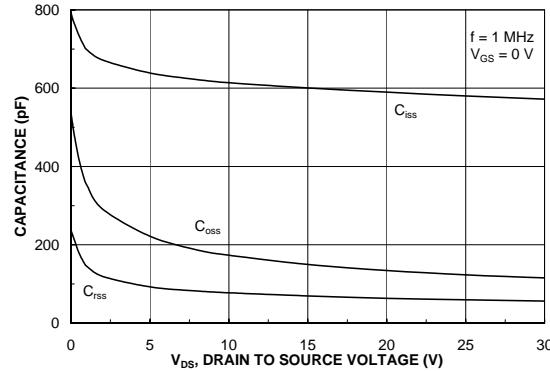
Figure 19. Capacitance Characteristics.
