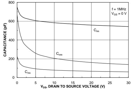
Figure 8. Capacitance Characteristics.
