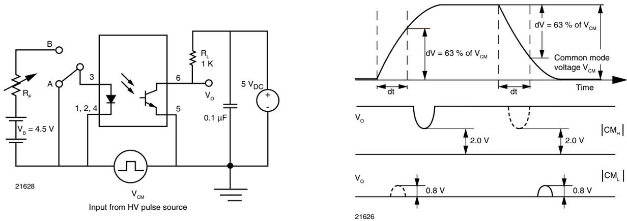
Fig. 3 - Test Circuit for Common Mode Transient Immunity
