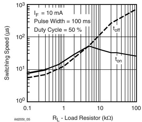
Fig. 8 - Switching Speed vs. Load Resistor
