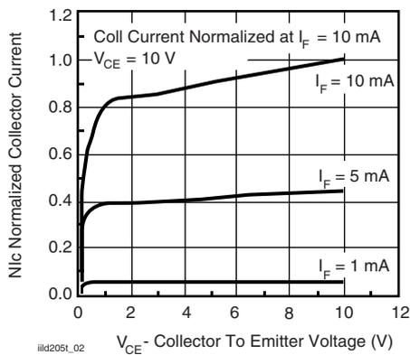
Fig. 5 - Collector Emitter Current vs. V<sub>CE</sub>
