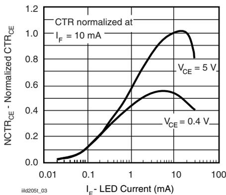
Fig. 6 - Normalized CTR<sub>CE</sub> vs. Forward Current
