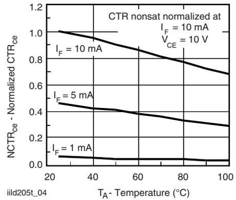
Fig. 7 - Current Transfer Ratio (normalized) vs. Ambient Temperature
