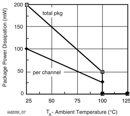
Fig. 1 - Power Dissipation vs. Ambient Temperature
