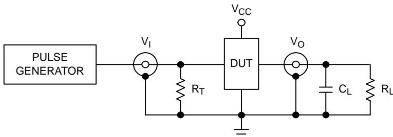
$C_L$  includes jig and probe capacitance
