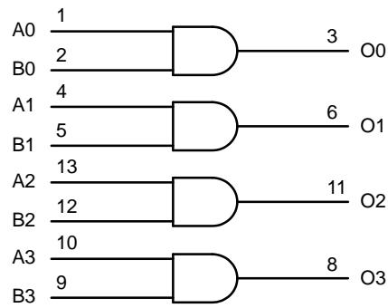
**Figure 2. Logic Diagram**
