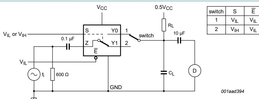
Fig. 17. Test circuit for measuring total harmonic distortion
