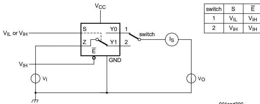
$V_I = V_{CC}$  or GND;  $V_O = \text{GND}$  or  $V_{CC}$ .
