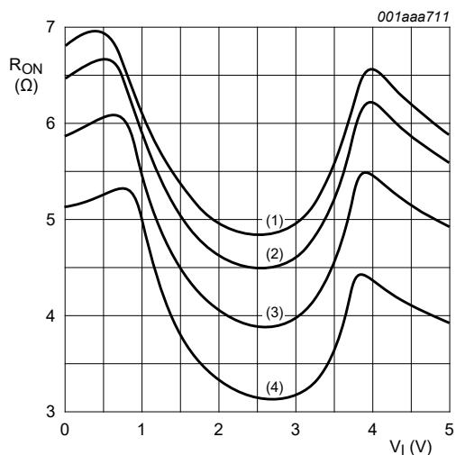
Fig. 13. ON resistance as a function of input voltage
