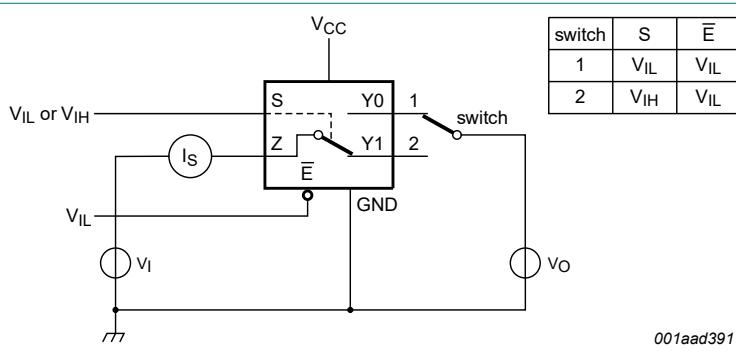
$V_I = V_{CC}$  or GND and  $V_O = \text{open circuit}$ .
