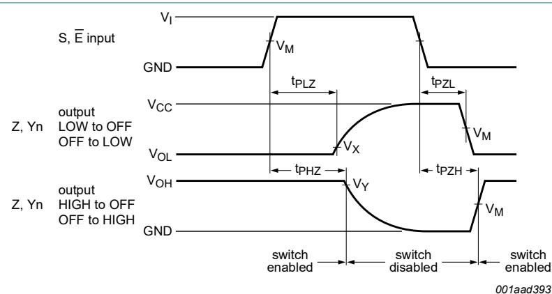
**Fig. 15. Enable and disable times**
