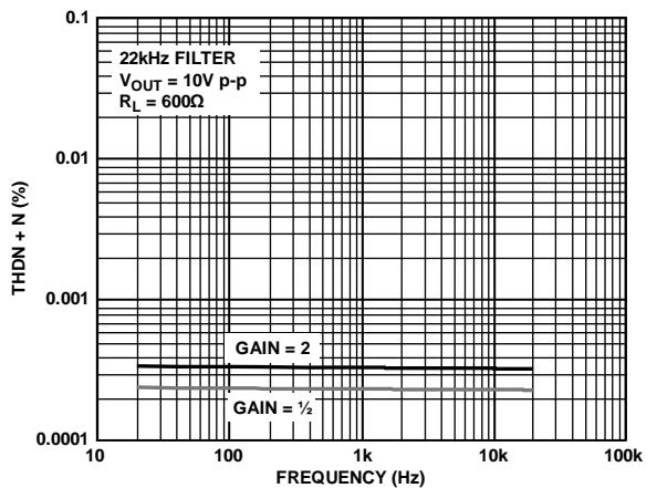
Figure 31. THD + N vs. Frequency, Filter = 22 kHz
