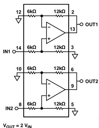
$V_{\text{OUT}} = 2 V_{\text{IN}}$
