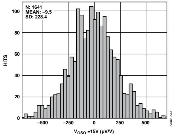
Figure 4. Typical Distribution of System Offset Voltage,
