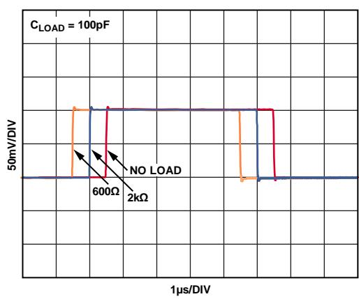
Figure 20. Small Signal Step Response, Gain = 2
