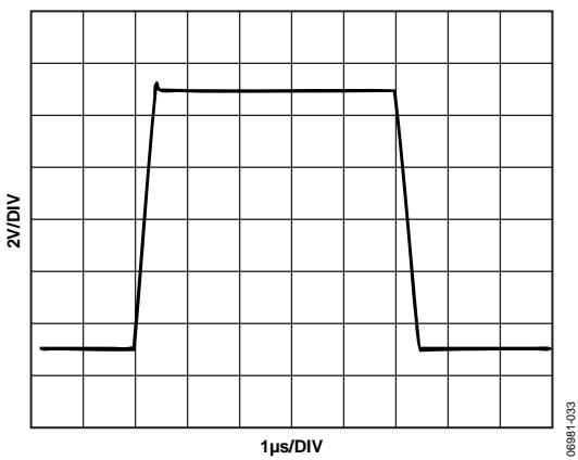
Figure 29. Large Signal Pulse Response, Gain = 2
