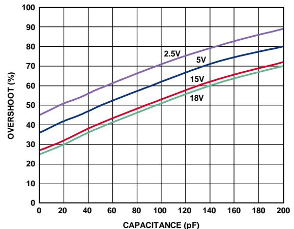
Figure 25. Small Signal Overshoot vs. Capacitive Load,  $G = \frac{1}{2}$ , 600 Ω in Parallel with Capacitive Load
