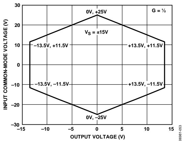
Figure 9. Input Common-Mode Voltage vs. Output Voltage,
