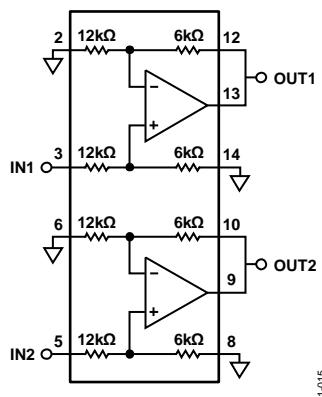
$V_{\text{OUT}} = \frac{1}{2} V_{\text{IN}}$
