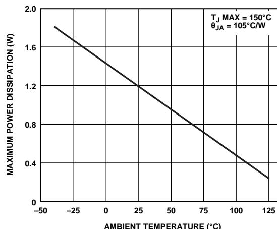
Figure 2. Maximum Power Dissipation vs. Ambient Temperature
