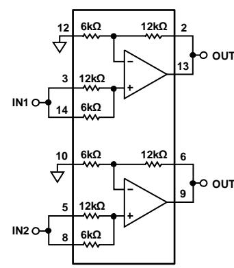
$V_{\text{OUT}} = 3 V_{\text{IN}}$
