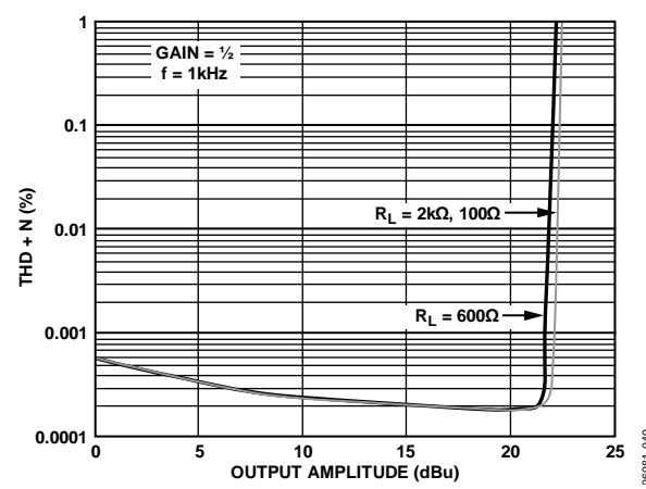
Figure 33. THD + N vs. Output Amplitude, G = 1/2
