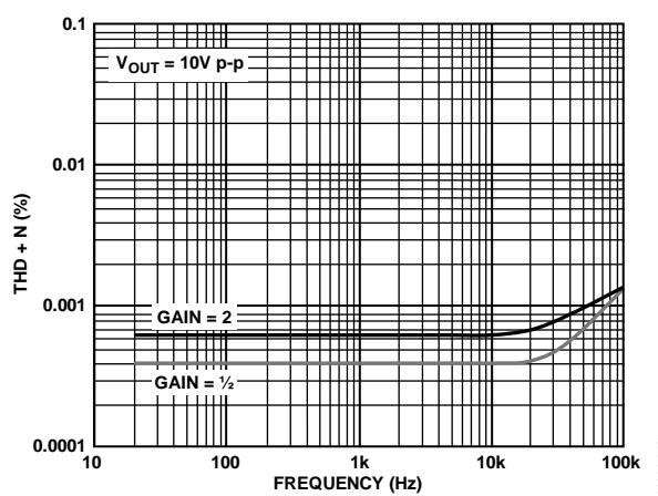
Figure 32. THD + N vs. Frequency, Filter = 120 kHz
