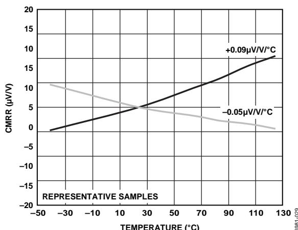
Figure 6. CMRR vs. Temperature, Normalized at 25°C
