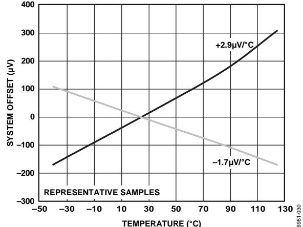
Figure 7. System Offset vs. Temperature, Normalized at 25°C,
