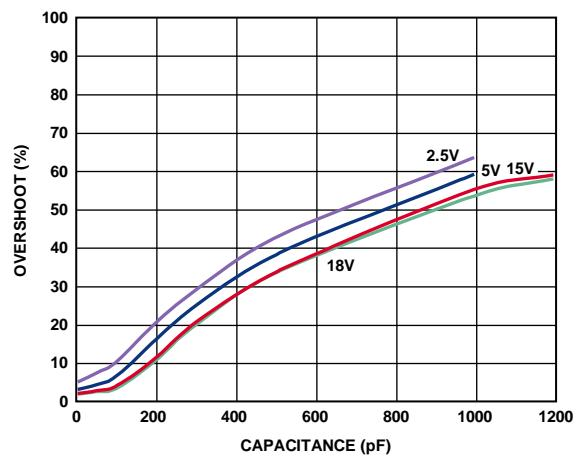
Figure 27. Small Signal Overshoot vs. Capacitive Load,  $G = 2$ , 600 Ω in Parallel with Capacitive Load
