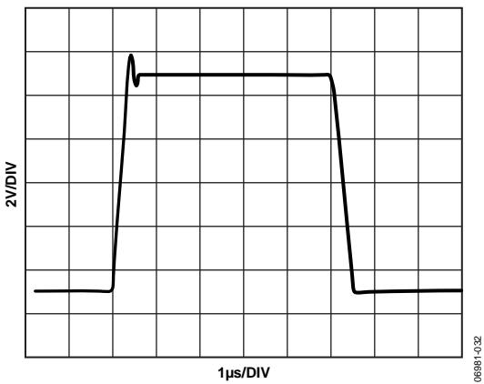
Figure 28. Large Signal Pulse Response, Gain = 1/2
