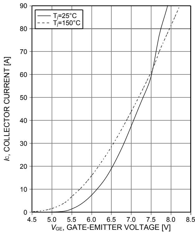
Figure 6. **Typical transfer characteristic**
