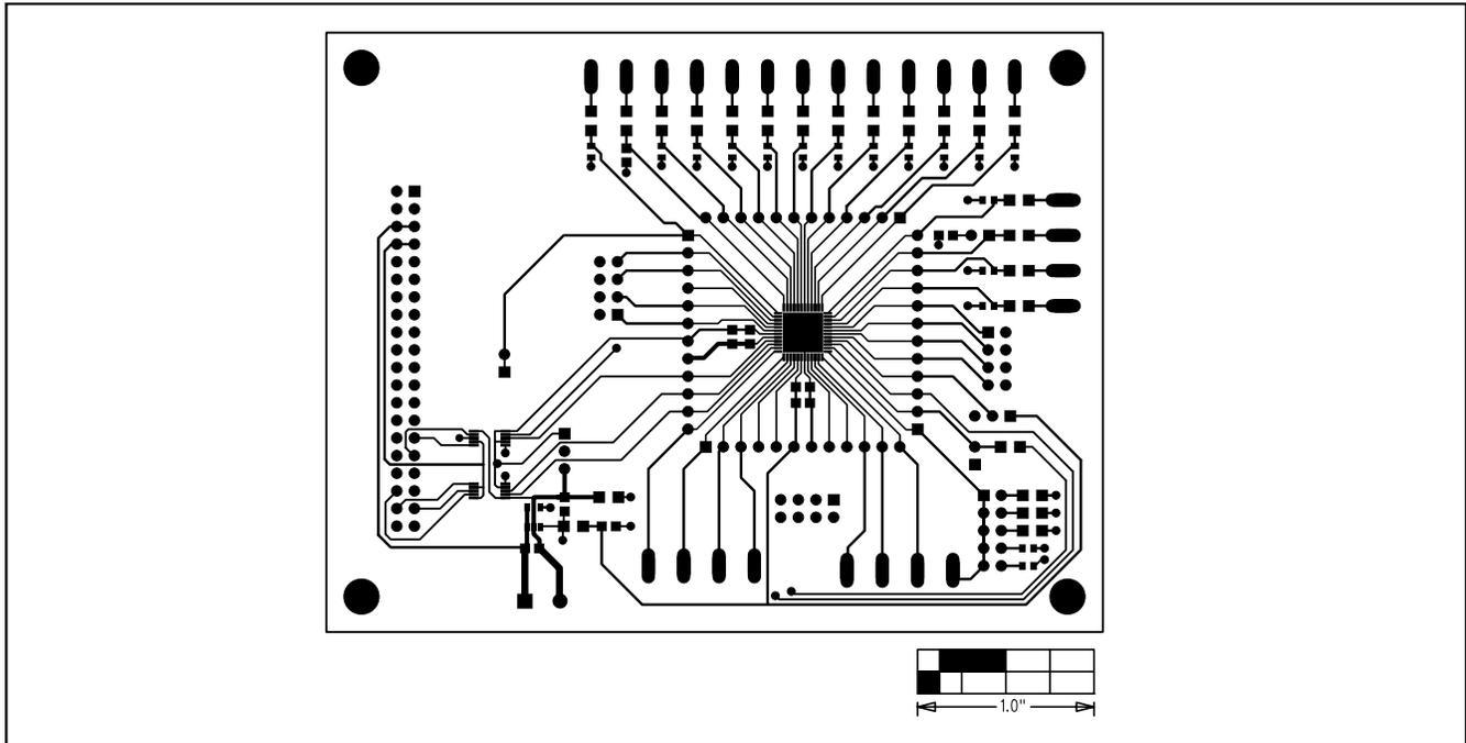
Figure 9. MAX1258 EV Kit PCB Layout—Component Side
