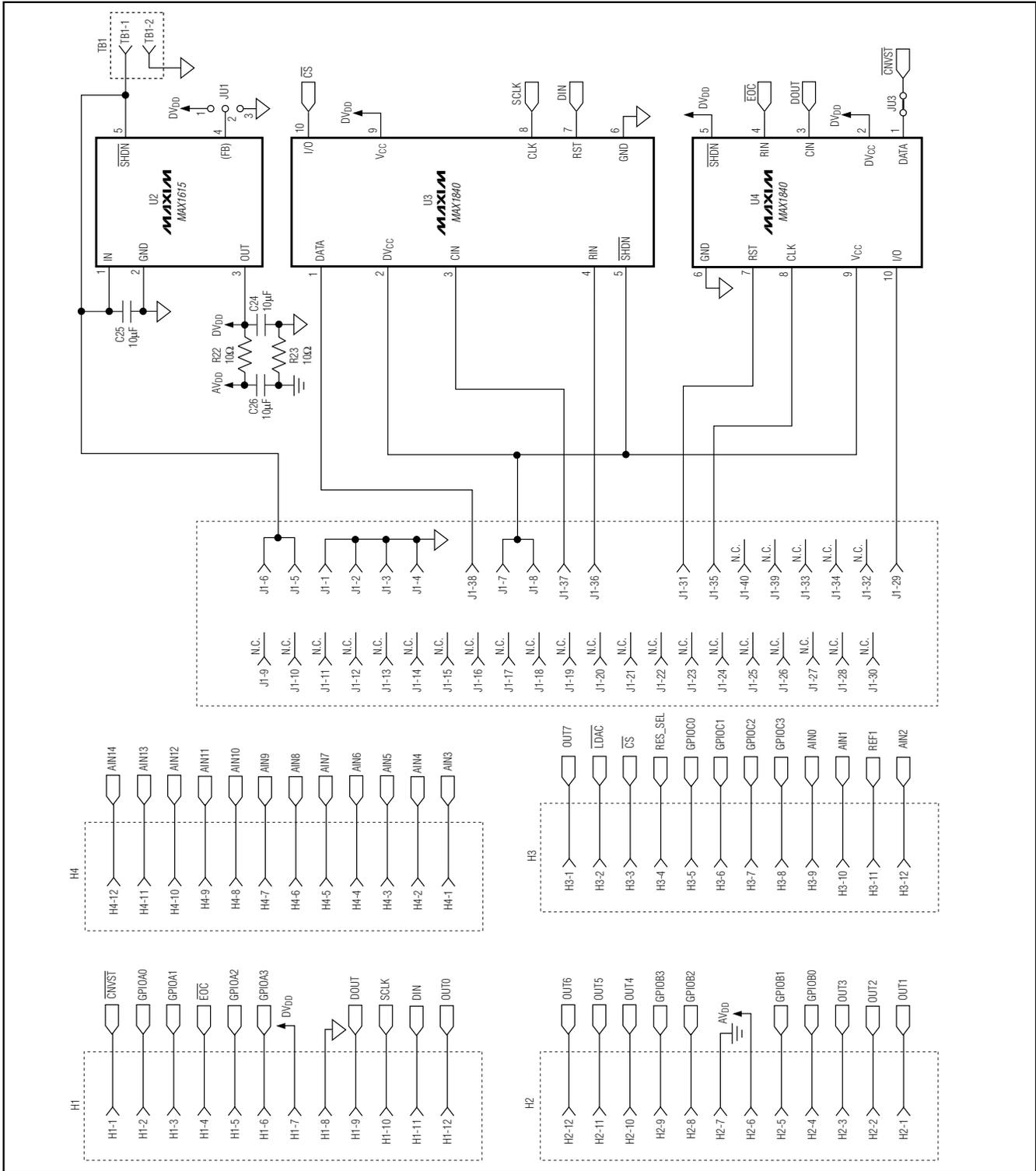
Figure 7b. MAX1258 EV Kit Schematic (Sheet 2 of 2)
