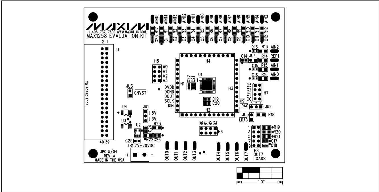
Figure 8. MAX1258 EV Kit Component Placement Guide—Component Side
