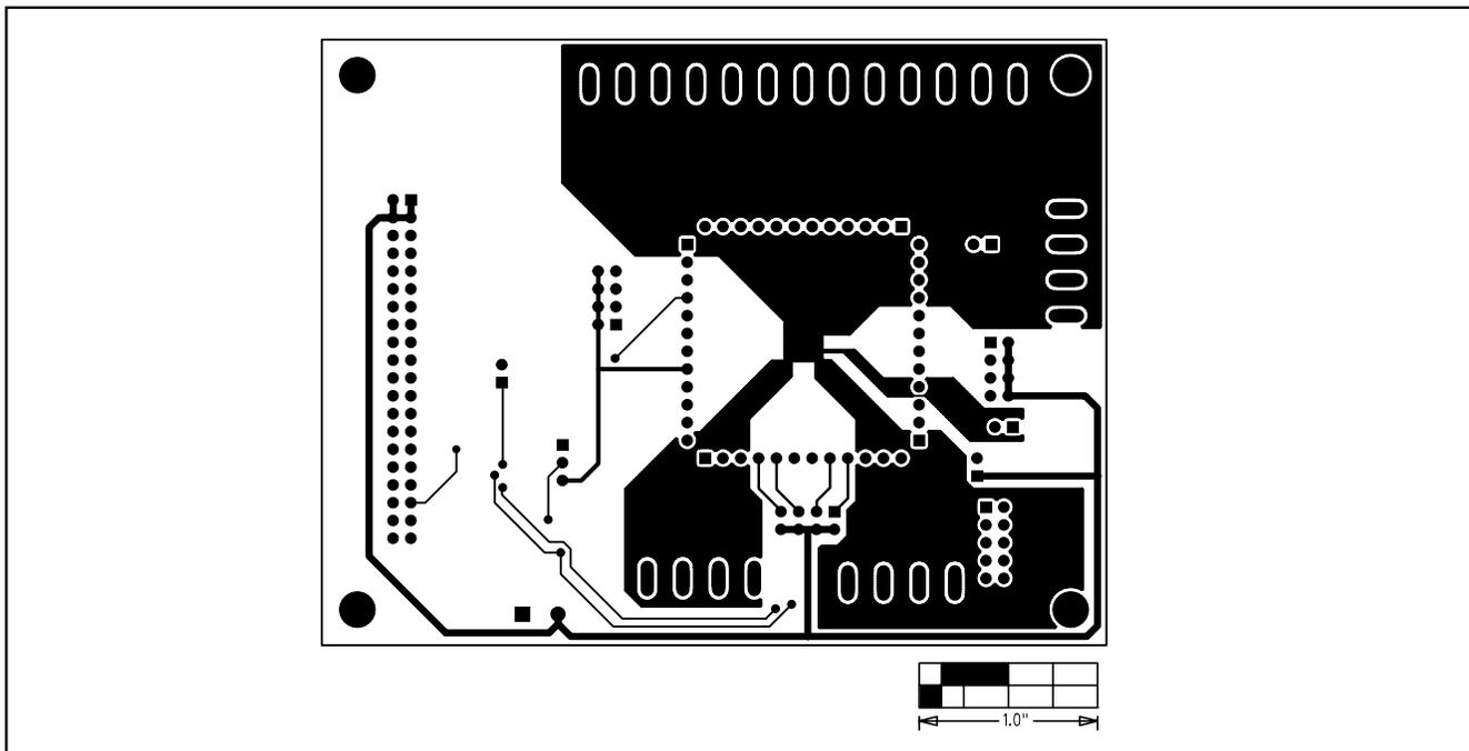
Figure 10. MAX1258 EV Kit PCB Layout—Solder Side
