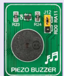
Figure 19-2: Use jumper J12 to connect Piezo buzzer on RDO or RA11 pin
