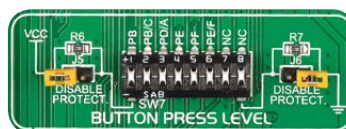
Figure 10-6: Button press level DIP switch (tri-state)
