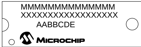
40-Lead CERDIP Windowed
