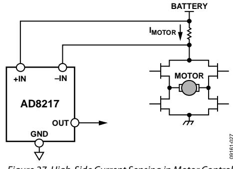
Figure 27. High-Side Current Sensing in Motor Control
