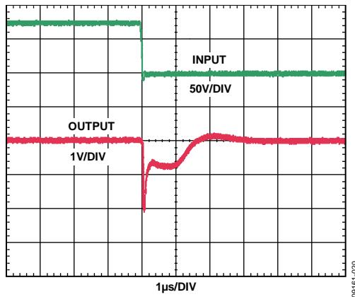
Figure 20. Common-Mode Step Response (Falling)
