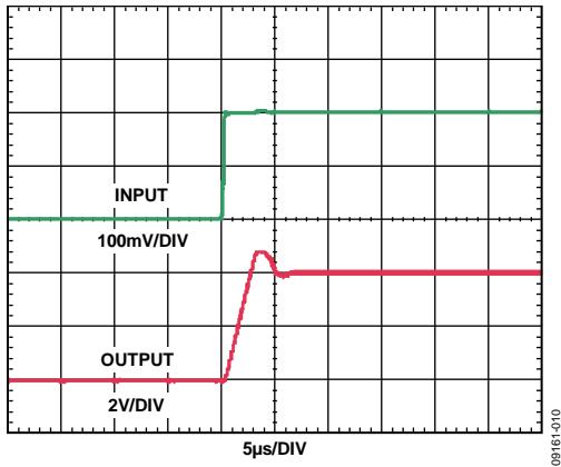
Figure 10. Rise Time (Differential Input = 200 mV)
