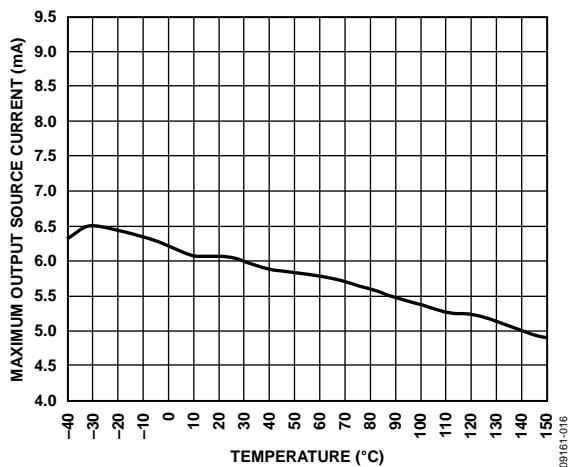
Figure 16. Maximum Output Source Current vs. Temperature
