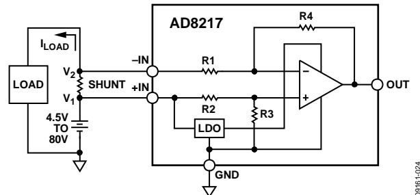
Figure 24. Simplified Schematic
