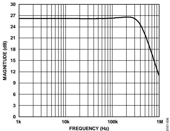
Figure 6. Typical Small-Signal Bandwidth ( $V_{out} = 200 \text{ mV p-p}$ )
