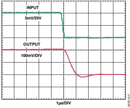
Figure 11. Fall Time (Differential Input = 5 mV)
