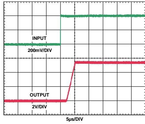
Figure 13. Differential Overload Recovery, Rising
