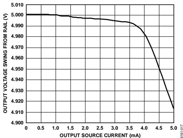
Figure 17. Output Voltage Range vs. Output Source Current
