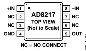
Figure 2. Pin Configuration
