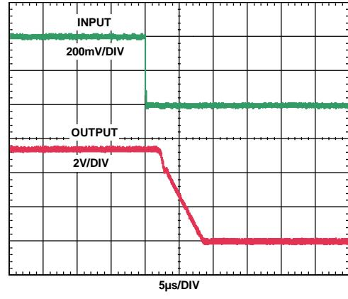
Figure 14. Differential Overload Recovery, Falling
