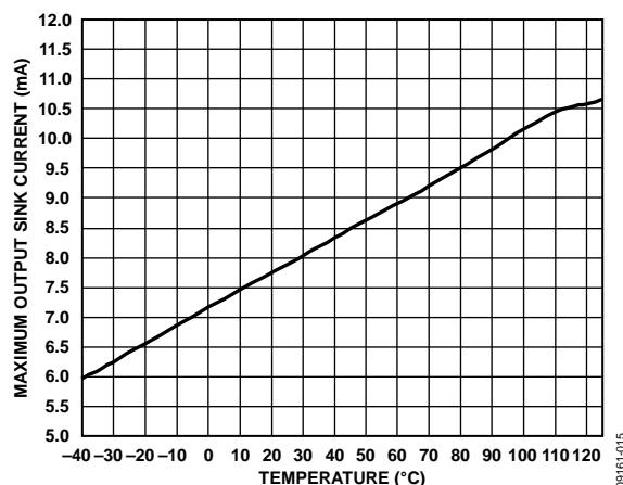
Figure 15. Maximum Output Sink Current vs. Temperature
