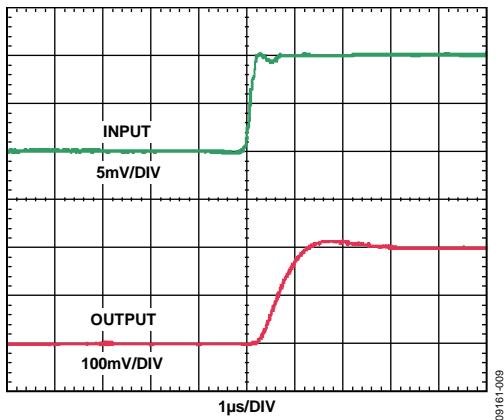
Figure 9. Rise Time (Differential Input = 5 mV)
