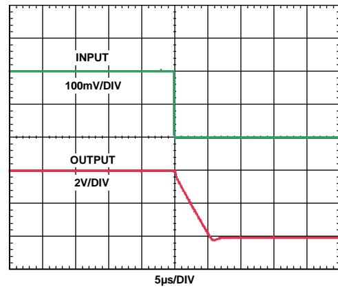
Figure 12. Fall Time (Differential Input = 200 mV)
