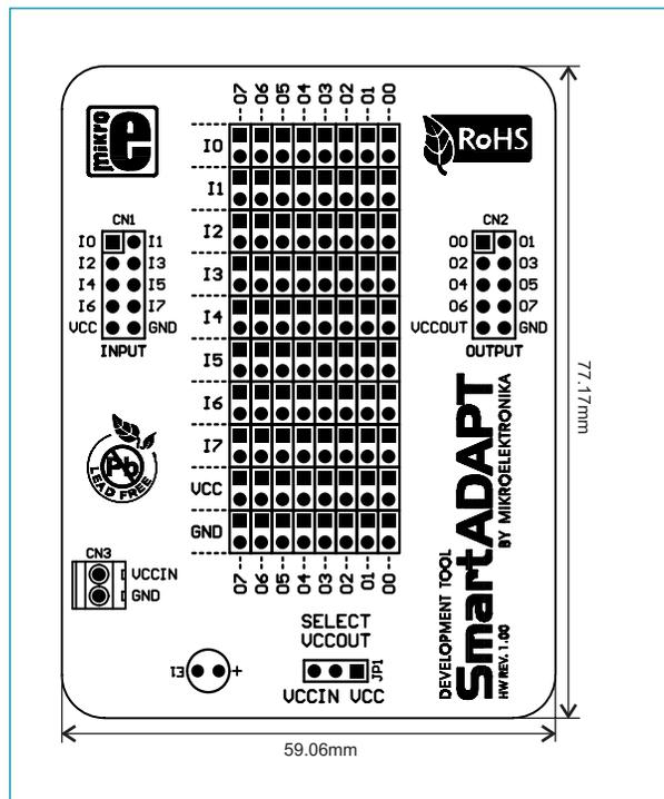
Figure 5: Dimensions of the Smart ADAPT board
