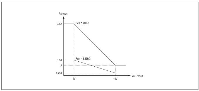
Figure 2. Startup Inrush Current Foldback Characteristics
