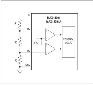
Figure 1. Undervoltage/Overvoltage-Threshold Setting
